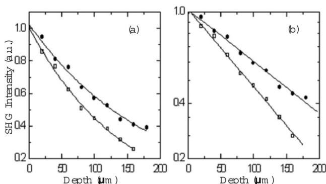
**Fig. 4** SHG signal of collagen. (a) SHG signal versus penetration depth for 800- (□) and 1300-nm (●) excitation wavelengths. The solid curves are a guide to the eye. (b) SHG intensities (logarithmic scale) versus penetration depth.
