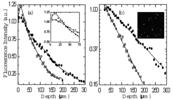
**Fig. 2** TPEF of fluorescent polystyrene beads in scattering agarose gels. (a) Fluorescent signal versus penetration depth for 800-nm ( $\square$ ) and 1300-nm ( $\bullet$ ) excitation wavelengths. The solid curves are a guide to the eye. (b) TPEF intensities (logarithmic scale) versus penetration depth for data starting from 25  $\mu\text{m}$ . Inset: image of the phantom at 15  $\mu\text{m}$  depth, using 1300-nm excitation wavelength.
