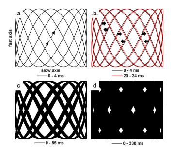
**Fig. 2** Calculated Lissajous scan patterns. Fast-axis frequency = 2219 Hz. Slow-axis frequency=986 Hz. (a) 0 to 4 ms, where the pattern nearly repeats itself. (b) A comparison of two Lissajous patterns 20 ms apart, showing how the pattern shifts over time. (c) 0 to 85 ms, showing partial coverage over the FOV. (d) 0 to 330 ms, showing nearly full coverage over the FOV.
