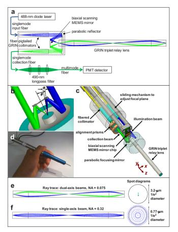
**Fig. 1** The GRIN-relayed DAC. (a) A schematic of the optical circuit of the microscope. (b) A close-up view of the parabolic focusing optic and the MEMS scanning mirror. (c) The microscope scan head and relay lens. (d) A photograph of the microscope exterior. (e) Ray-trace and spot diagrams of the dual-axis illumination (blue) and collection (green) beam paths within a GRIN relay lens. (f) Ray-trace and spot diagrams of a single large-NA GRIN-relayed beam. (Color online only.)
