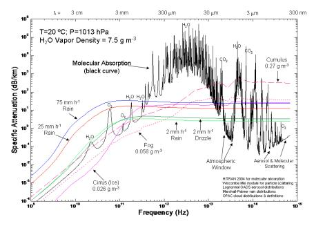
Fig. 1. Specific attenuation from 30 cm to  $\sim$ 0.4  $\mu$ m (1 GHz to 750 THz). The black line is molecular absorption with some effects of continent average aerosols and molecular scattering included. Colored lines represent the specific attenuation that would be added for the hydrometeor distributions shown (rain, clouds, fog).
