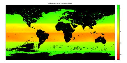
Fig. 9. Worldwide SNR values for 1.557  $\mu$ m (Top), 95 GHz (Middle), and 250 GHz (Bottom), January, 50th percentile RH, daily average, molecular and aerosol effects plus stratus layer between 500 m and 1000 m, 1530 m slant range, near-vertical path, 1525 m platform altitude. Note different color scales.
