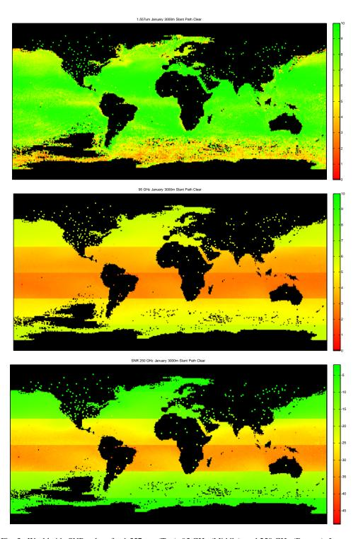
Fig. 3. Worldwide SNR values for 1.557  $\mu m$  (Top), 95 GHz (Middle), and 250 GHz (Bottom), January, 50th percentile RH, daily average, no cloud, molecular and aerosol effects only, 3000 m slant range, oblique path, 1525 m platform altitude. Note different color scales.
