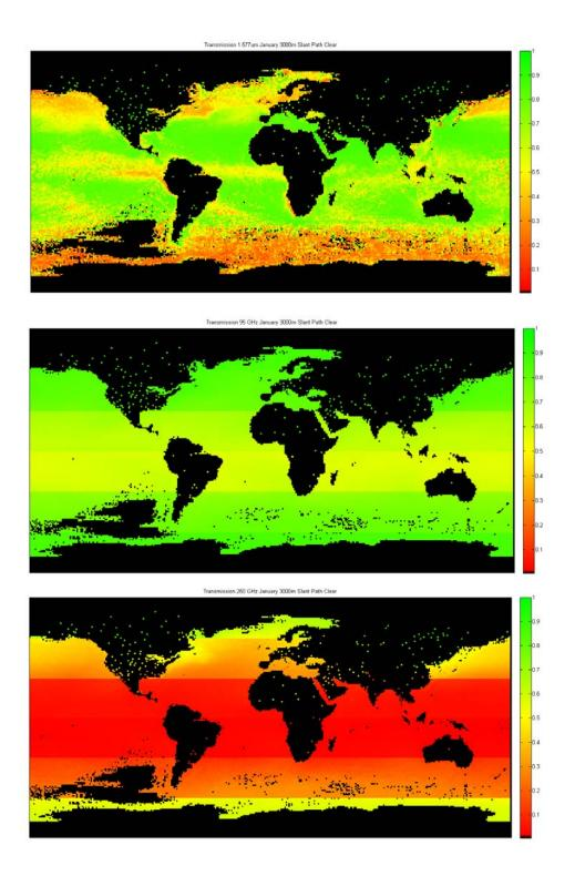
Fig. 2. Worldwide path transmittance values for the climatological atmosphere for 1.557  $\mu$ m (Top), 95 GHz (Middle), and 250 GHz (Bottom), for January, 50th percentile RH, daily average, molecular and aerosol effects, 3000 m slant range, oblique path, 1525 m platform altitude.
