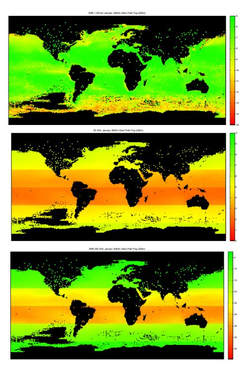
Fig. 6. Worldwide SNR values for 1.557  $\mu$ m (Top), 95 GHz (Middle), and 250 GHz (Bottom), January, 50th percentile RH, daily average, molecular and aerosol effects plus 200 meter fog layer, 3000 m slant range, oblique path, 1525 m platform altitude. Note different color scales.
