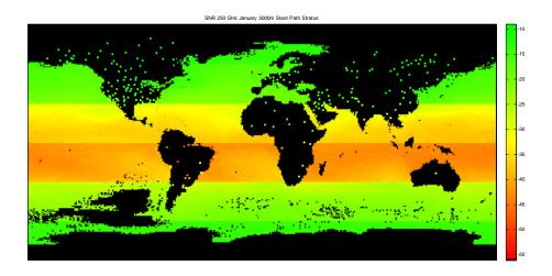
Fig. 8. Worldwide SNR values for 1.557  $\mu$ m (Top), 95 GHz (Middle), and 250 GHz (Bottom), January, 50th percentile RH, daily average, molecular and aerosol effects plus stratus layer between 500 m and 1000 m, 3000 m slant range, oblique path, 1525 m platform altitude. Note different color scales.
