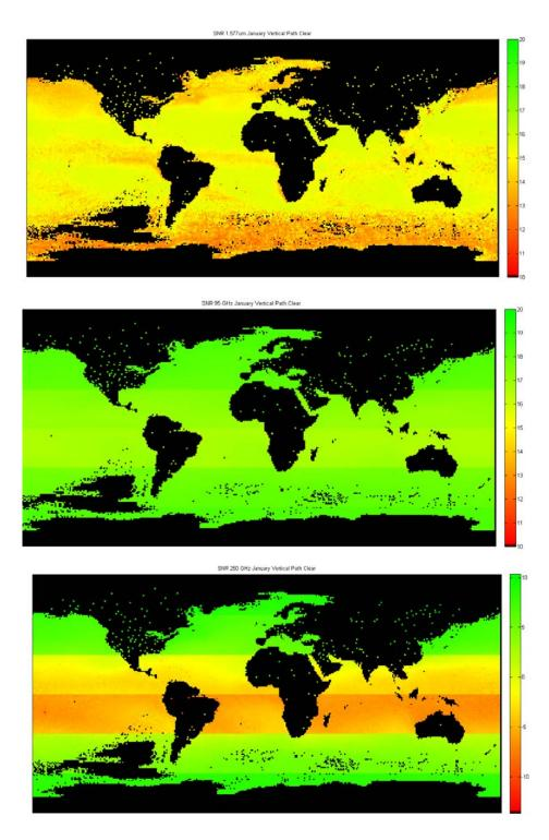
Fig. 4. Worldwide SNR values for 1.557  $\mu$ m (Top), 95 GHz (Middle), and 250 GHz (Bottom), January, 50th percentile RH, daily average, no cloud, molecular and aerosol effects only, 1530 m slant range, 1525 m platform altitude, near-vertical path. Note different color scales.
