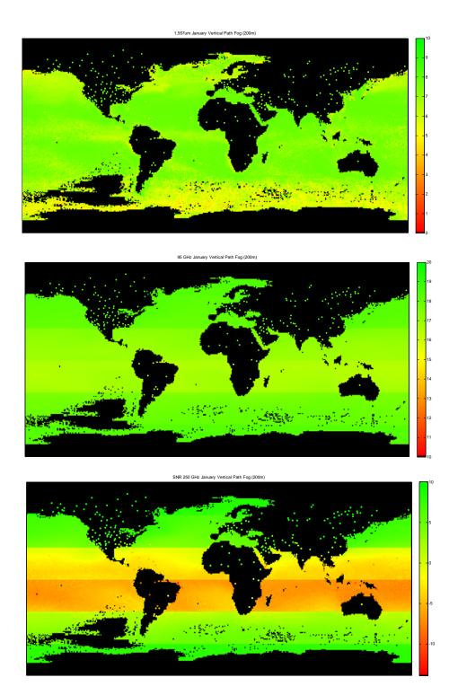
Fig. 7. Worldwide SNR values for 1.557  $\mu$ m (Top), 95 GHz (Middle), and 250 GHz (Bottom), January, 50th percentile RH, daily average, molecular and aerosol effects plus 200 meter fog layer, 1530 m slant range, 1525 m platform altitude, near-vertical path. Note different color scales.
