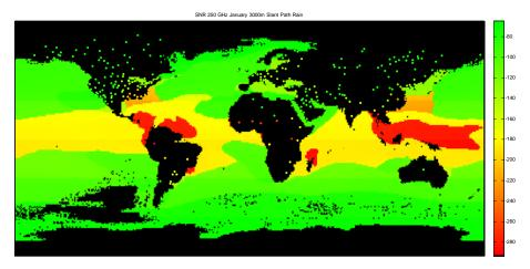
Fig. 11. Worldwide SNR values for 1.557 μm (Top), 95 GHz (Middle), and 250 GHz (Bottom), January, 50th percentile RH, daily average, molecular and aerosol effects, plus locally heavy rain (99.98th percentile), 3000 m slant range, 1525 m platform altitude. Note different color scales.
