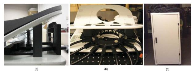
Fig. 1 (a) Biopsy plate slab interface with slots for fibers, (b) circular breast interface containing optical fibers shown positioned in the MR breast coil, and (c) integrated mobile cart containing the NIR data collection instrumentation.
