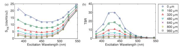
**Fig. 10** Measured (symbols) and calculated (dashed lines) (a) capillary signal versus  $\lambda_{ex}$  and (b) the corresponding TBR versus  $\lambda_{ex}$  curves at Z = 6X for the 20% phantoms. Almost identical results were obtained at Z = 3X (data not shown).
