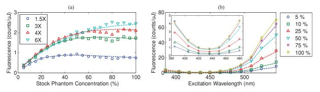
**Fig. 8** Monte Carlo calculations (dashed lines) and experimental measurements (symbols) in the liquid phantoms. (a) AF versus *C* for various zoom factors (*Z* = 1.5, 3, 4, 6X) at  $\lambda_{ex} = 465$  nm and  $\lambda_{ex} = 600$  nm. (b) AF versus  $\lambda_{ex}$  for various concentrations (*C* = 5, 10, 25, 50, 75, 100%) at *Z* = 6X and  $\lambda_{ex} = 600$  nm. The insert shows the low signal region re-scaled for better viewing. The Monte Carlo results were normalized at  $C_0 = 40\%$ .
