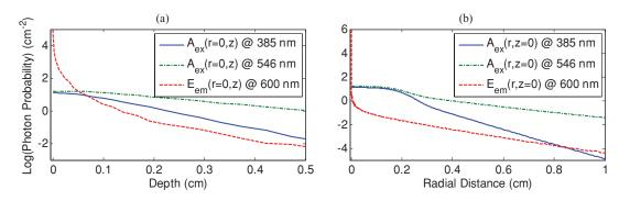
**Fig. 5** Typical Monte Carlo results for (a) depth-resolved and (b) radial excitation fluence  $Y_{ex}(r,z)$  (solid and dotted lines) and escape function  $E_{em}(r,z)$  (dashed lines) for the 20% phantom sample at 3X zoom. For this particular sample the optical properties were  $\mu_a = 4.97$ , 0.57, 1.77 cm<sup>-1</sup> and  $\mu'_s = 7.81$ , 5.94, 5.42 cm<sup>-1</sup> at 385, 546 and 600 nm, respectively.
