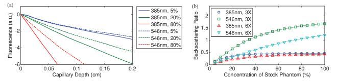
Fig. 6 Typical Monte Carlo results for (a) the detected target signal versus capillary depth  $F_{ex,em}(z_c)$  and (b) the backscattering ratio calculated for the liquid phantoms  $R_{ex,C}$  versus C.
