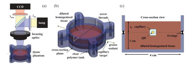
Fig. 1 Experimental design: (a) epifluorescence imaging setup, (b) tank designed for the inclusion of a capillary target in liquid phantoms, (c) cross-section view.
