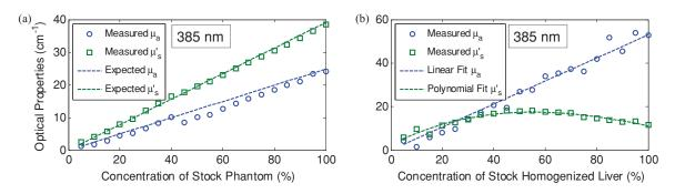
Fig. 7 Optical properties versus C, showing both measured data (symbols) and either expected or fitted values (lines), for (a) the liquid phantoms and (b) the liver homogenate.
