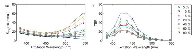
**Fig. 9** Measured (symbols) and calculated (dashed lines) (a) surface capillary signal,  $X_{TR0}$  versus  $\lambda_{ex}$  and (b) the corresponding TBR versus  $\lambda_{ex}$  results obtained at Z = 6X for various phantom concentrations (C = 5, 10, 15, 20, 40, 60, 80%). The black solid line in (a) represents the corrected background-free quantum dot fluorescence,  $UX'_{OD0}$ . Almost identical results were obtained at Z = 3X (data not shown).
