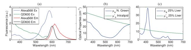
Fig. 2 (a) Fluorescence excitation (dashed lines) and emission (solid lines) spectra of QD600 and AlexaFluor 568. (b) Optical properties of the main absorber (Naphthol Green, dashed line) and scatterer (Intralipid 20%, solid line) for the stock (100%) liquid phantom. (c) Measured optical properties of the 25% liver homogenate.
