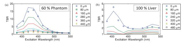
Fig. 13 Proof-of-principle Monte Carlo evaluation of TBR data to unreachable experimental conditions. (a) for very shallow depths and (b) for nondiluted tissue.
