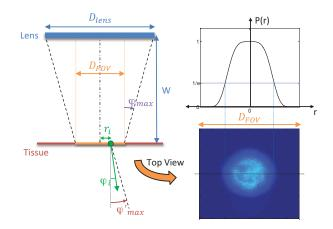
**Fig. 4** Illumination geometry for epifluorescence imaging (left) and the excitation profile used in the Monte Carlo model. The values of  $D_{FOV}$  were 1.45, 0.8, 0.6, and 0.4 cm at Z = 1.5, 3, 4, 6X.
