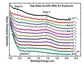
**Fig. 8** Near HOMO region UPS data for 50 Å MoO<sub>x</sub> and  $10^2$ ,  $10^4$ ,  $10^6$ ,  $10^8$ ,  $10^{10}$ ,  $10^{11}$ ,  $10^{12}$ ,  $5 \times 10^{12}$ ,  $10^{13}$ ,  $5 \times 10^{13}$ ,  $10^{14}$ , and  $2 \times 10^{14}$  L air exposure.
