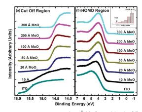
**Fig. 4** UPS data for 300, 200, 100, 50, 20, and 10 Å MoO<sub>x</sub> and *in situ* OP-treated ITO for (a) the cutoff region and (b) the HOMO region. Inset: Schematics of gradual thickness of  $MoO_x$ .
