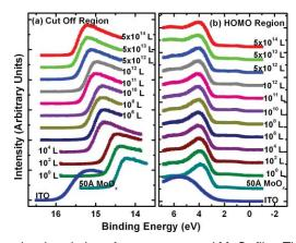
**Fig. 9** Electronic energy-level evolution of oxygen-exposed MoO<sub>x</sub> film. The UPS data presented is for ITO, 50 Å MoOx, and 1, 10<sup>2</sup>, 10<sup>4</sup>, 10<sup>6</sup>, 10<sup>8</sup>, 10<sup>10</sup>, 10<sup>11</sup>, 10<sup>12</sup>, 5 × 10<sup>12</sup>, 5 × 10<sup>13</sup>, and 5 × 10<sup>14</sup> L oxygen exposure (a) the cutoff region and (b) the HOMO region. Continuous reduction in surface WF is demonstrated.
