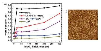
**Fig. 5** (a) Work function versus MoO<sub>x</sub> interlayer thickness for 4 Å ( $\bullet$ ), 8 Å ( $\blacktriangle$ ), 32 Å ( $\blacktriangledown$ ) and 128 Å ( $\blacklozenge$ ) AIPc-CI coverages. (b) AFM data for 2 × 2 $\mu$ m area of 228-Å-thick AIPc-CI film.
