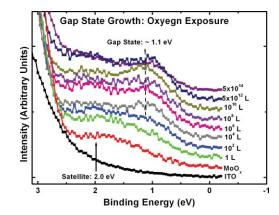
**Fig. 11** Near HOMO region UPS data *in situ* OP-treated ITO, 50 Å MoOx, and 1, 10<sup>2</sup>, 10<sup>4</sup>, 10<sup>6</sup>, 10<sup>8</sup>, 10<sup>10</sup>,  $5 \times 10^{12}$ , and  $5 \times 10^{14}$  L oxygen exposure. The growth of gap state at ~1.1 is clearly visible.
