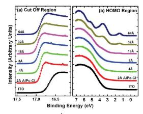
Fig. 1 UPS data for 64, 32, 16, 8, 4, and 2 Å AIPc-CI and ITO for (a) the cutoff region and (b) the HOMO region.
