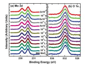
**Fig. 7** XPS data for, (a) the Mo 3d and (b) the O 1s core level for, ITO, 50 Å MoO<sub>x</sub>, and 10<sup>2</sup>, 10<sup>4</sup>, 10<sup>6</sup>, 10<sup>8</sup>, 10<sup>10</sup>, 10<sup>11</sup>, 10<sup>12</sup>,  $5 \times 10^{12}$ ,  $10^{13}$ ,  $5 \times 10^{13}$ ,  $10^{14}$ , and  $2 \times 10^{14}$  L air exposure.
