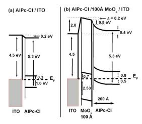
**Fig. 3** The energy level alignment at AIPc-CI/ITO interface (a) without and (b) with 100 Å  $MoO_x$  insertion layer. Strong band bending is observed in the presence of the  $MoO_x$  interlayer between ITO and AIPc-CI.
