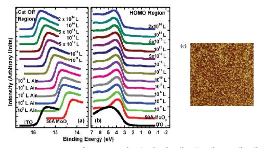
**Fig. 6** UPS data for ITO; 50 Å MoO<sub>x</sub>; and 10<sup>2</sup>, 10<sup>4</sup>, 10<sup>6</sup>, 10<sup>8</sup>, 10<sup>10</sup>, 10<sup>11</sup>, 10<sup>12</sup>,  $5 \times 10^{12}$ , 10<sup>13</sup>,  $5 \times 10^{13}$ ,  $10^{14}$ , and  $2 \times 10^{14}$  L air exposure in (a) the cutoff region and (b) the HOMO region. Substantial to low WF reduction is observed, depending on the amount of air exposure. (c) AFM image of 50-Å MoO<sub>x</sub> film is presented.
