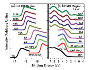
**Fig. 2** Electronic energy-level evolution (UPS data) for 228, 128, 64, 32, 16, 8, 4, and 2 Å AlPc-Cl, and ITO with 100 Å MoO<sub>x</sub> interlayer for (a) the cutoff region and (b) the HOMO region.
