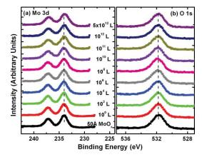
**Fig. 10** Core energy-level evolution of MoO<sub>x</sub> film. XPS data for, (a) the Mo 3d and (b) the O 1s core level for, ITO, 50 Å MoO<sub>x</sub>, and 1, 10<sup>2</sup>, 10<sup>4</sup>, 10<sup>6</sup>, 10<sup>8</sup>, 10<sup>10</sup>, 10<sup>11</sup>, 10<sup>12</sup>,  $5 \times 10^{12}$ ,  $5 \times 10^{13}$ , and  $5 \times 10^{14}$  L oxygen exposure.
