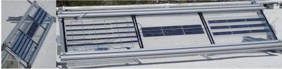
**Fig. 2** Experimental setup for the measurement of the cell temperature of the DA holographic panels. The coupons had the following arrangement: (left) 2 to 1 holographic coupon: (middle) packed reference coupon: (right) 1 to 1 holographic coupon. The system was pointed south and tilted for latitude.
