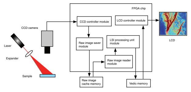
Fig. 3 The main architecture of the SOC solution for the LSI system. The direction of the arrow stands for the direction of the data that flows in the main modules.
