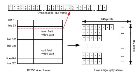
Fig. 4 Extracting the Y components (gray scale value) from BT656 video frame to make up a raw image that can be used to perform LSI processing.
