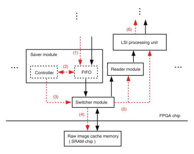
Fig. 5 The architecture for sharing the raw image cache memory by saver module and reader module. The red dashed line arrows stand for the handshaking signal or control signal. The black solid line arrows stand for data signal. The direction of the arrow stands for the transferring direction of the handshaking signal, control signal, and data. The red number in the bracket is used to mark the nearby handshaking signal or control signal.
