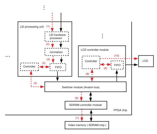
**Fig. 6** The architecture of operating the video memory by a LSI processing unit module and LCD controller module. The red dashed line arrows stand for the handshaking signal or control signal. The black solid line arrows stand for the data signal. The direction of the arrow stands for the transferring direction of the handshaking signal, control signal, and data. The red number in the bracket is used to mark the nearby handshaking signal or control signal.
