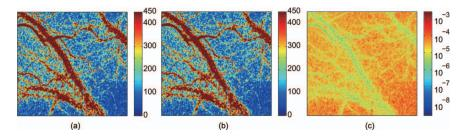
**Fig. 7** The LSI blood flow map of the mouse cerebral cortex processed in a different platform and comparison: (a) The LSI blood flow map processed by a LSI hardware processor in FPGA; (b) the LSI blood flow map processed by a program written in C + + running on a personal computer with single precision; (c) the relative difference map in logarithm format between image (a) and image (b).
