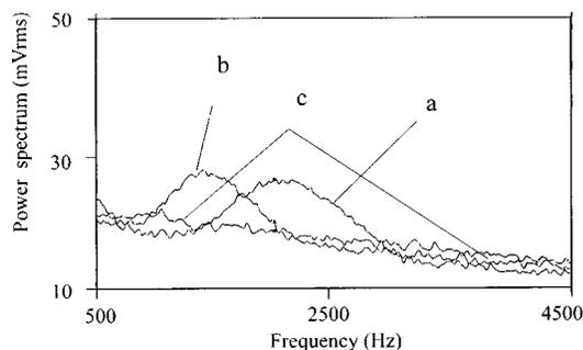
**Fig. 4** Doppler frequency shift spectra from a rotating disc with a pulsing R6G dye Nd:YLF pumped laser (source S3). Laser pulse duration is 5–8 ps, repetition rate 3.8 MHz. Plot (a) corresponds to the velocity of the scattering surface of the disc  $V=4.8$  mm/s; plot (b)  $V=3.2$  mm/s; plot (c) unmoving disc.
