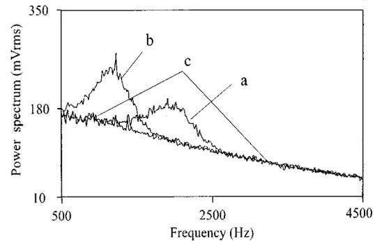
**Fig. 2** Doppler frequency shift spectra from a rotating disc with a pulsing diode laser (source S1). Laser pulse duration is 300 ns, repetition rate 700 kHz. Plot (a) corresponds to the velocity of the scattering surface of the disc  $V = 4.8$  mm/s; plot (b)  $V = 3.2$  mm/s; plot (c) unmoving disc.
