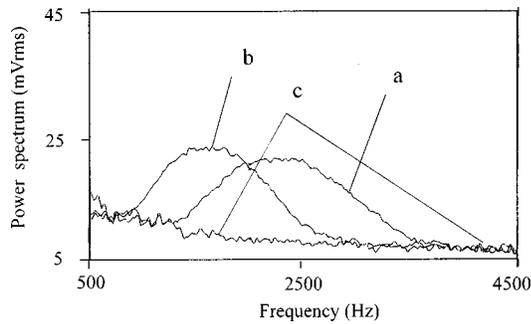
**Fig. 3** Doppler frequency shift spectra from a rotating disc with a pulsing Nd:YLF laser (source S2). Laser pulse duration is 35 ps, repetition rate 76 MHz. Plot (a) corresponds to the velocity of the scattering surface of the disc  $V=7.2$  mm/s; plot (b)  $V=4$  mm/s; plot (c) unmoving disc.
