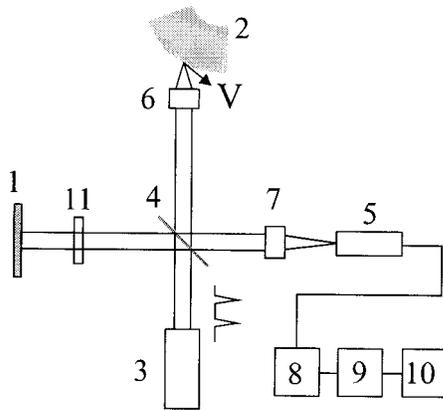
**Fig. 1** The scheme of the laser Doppler heterodyne flowmeter with an ultrashort pulsing laser source.
