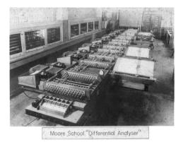
**Fig. 2** Mechanical computer used with J. G. Brainerd in 1939 to solve the nonlinear differential equations representing enzyme-substrate kinetics at the Moore School of Engineering at the University of Pennsylvania.
