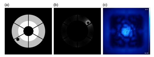
**Fig. 19** (a) Input pupil with seven misaligned segments in flower configuration. (b) Corresponding distribution of light in the Lyot stop plane for the RAVC. (c) Averaged noiseless coronagraphic PSF in the presence of atmospheric turbulence.
