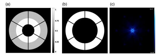
**Fig. 1** Illustration of the RAVC design for METIS, showing the input pupil (circularized version of the ELT pupil) with its (a) grayscale apodizer, (b) the Lyot stop, and (c) the associated theoretical PSF for the charge-2 RAVC on a field of view of  $100\lambda/D$ .
