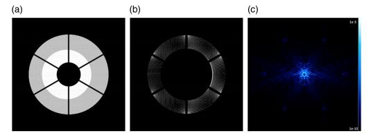
**Fig. 21** Effect of the ring apodizer misalignment on the RAVC behavior. The misalignment has been exaggerated to 5% here for the sake of illustration. Illustration of (a) the apodizer, (b) intensity distribution at the Lyot plane just after the Lyot stop, and (c) associated coronagraphic PSF.
