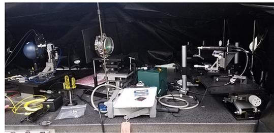
**Fig. 9** (a) The dispersion scale measurement set up and (b) the photo of the set up. The grism tips and tilts to simulate the desired field position.
