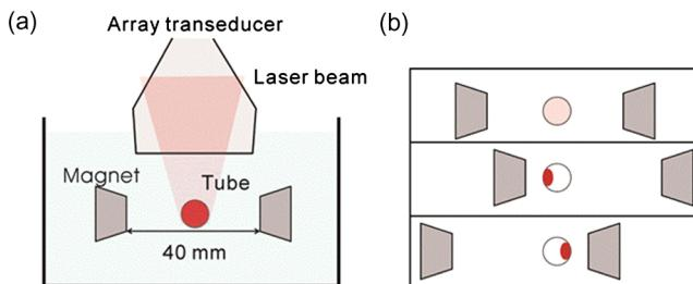
**Fig. 3** (a) Experimental setup of the mmPA imaging system. (b) Translation of the magnet system for dynamic magnetic manipulation of GMSNP. (Color online only.)
