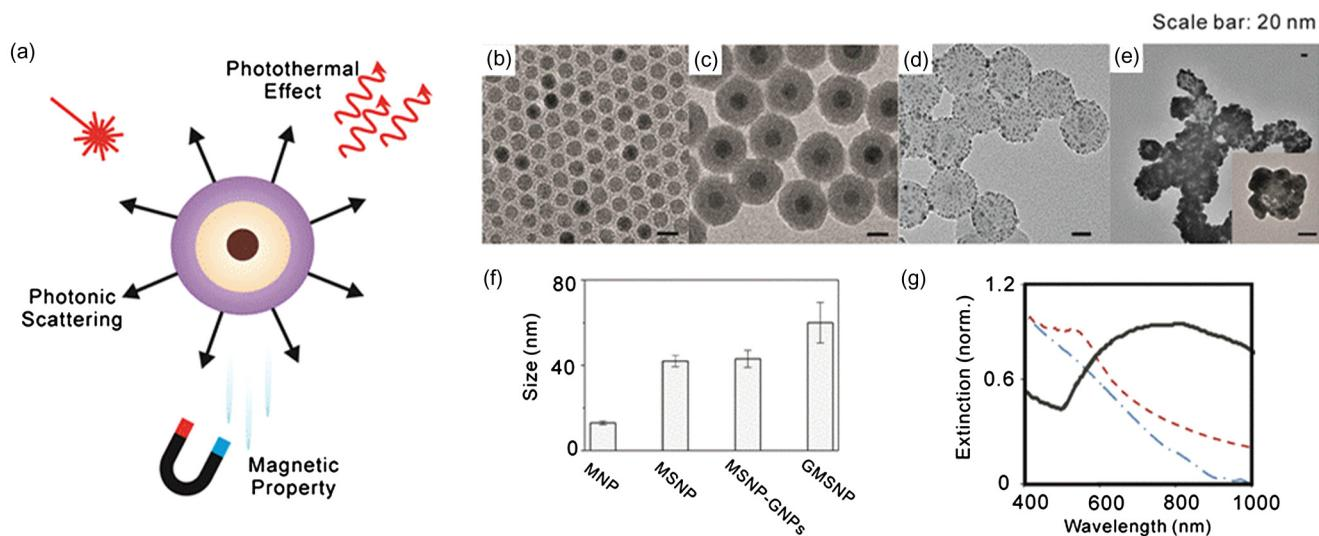
**Fig. 4** (a) Illustration of the multifunctional properties of GMSNP as a contrast agent for optical imaging techniques. Transmission electron microscopy images of (b) MNP, (c) MSNP, (d) MSNP-GNRs (e) GMSNP. (f) The size distribution of each nanoparticle. (g) UV-Vis-NIR extinction of MNP, MSNP and GMSNP. The characteristic absorbance of GMSNP is red-shifted due to the outer gold shell. (Color online only.)
