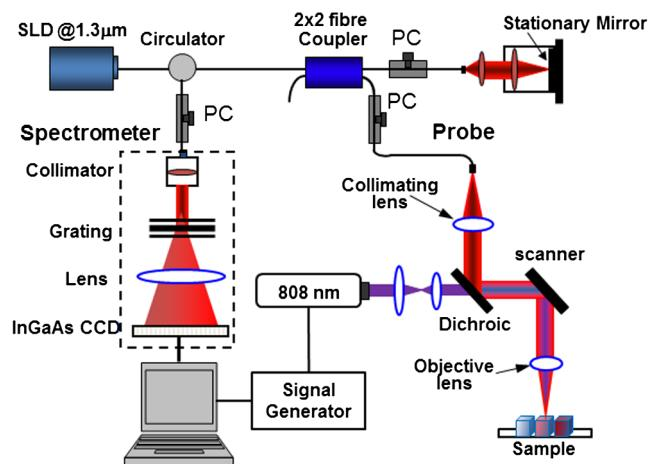
**Fig. 2** Schematic illustration of photothermal OCT for imaging GMSNP. (Color online only.)
