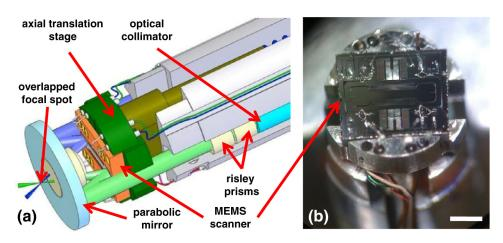
**Fig. 1** A 5.5-mm diameter DAC microendoscope scanhead. (a) Two collimated beams are focused by a parabolic mirror. Real-time *en face* scanning is performed by a 2-D MEMS scanner. (b) Photograph of the microendoscope without its cap showing a 2-D MEMS scanner mounted on the axial translation stage; Scale bar = 3 mm.
