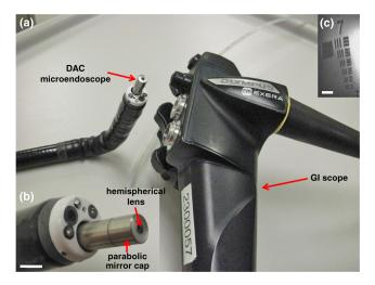
**Fig. 2** (a) A DAC microendoscope is passed through the instrument channel of an Olympus XT-160 endoscope that has a 6-mm diameter instrument channel. (b) Distal end of an endoscope showing the protruding DAC microendoscope; Scale bar = 5 mm. (c) Cropped reflectance image of a 1951 United States Air Force resolution test chart collected using the DAC microendoscope. Shows a transverse resolution of 5  $\mu$ m; Scale bar = 20  $\mu$ m.
