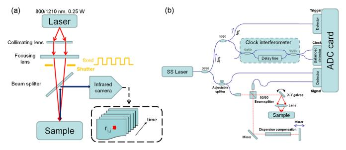
Fig. 2 Schematic diagrams of (a) PTW imaging instrumentation to measure the IR signal from plaques in response to periodic laser irradiation (800 and 1210 nm); and (b) intensity OCT system to measure plaque surface structure ("SS": swept source).
