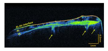
**Fig. 3** OCT images of the adhesion process on dentin using DBAs prepared with gold nanoparticles. The adhesion process regions are identified: adhesive layer (AL), hybrid layer (HL), and resin tags (arrows).
