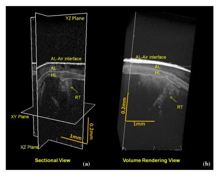
Fig. 4 Three-dimensional reconstruction with (a) sectional and (b) volume rendering views. The adhesive layer (AL), hybrid layer (HL), and resin tags (RT) are identified.
