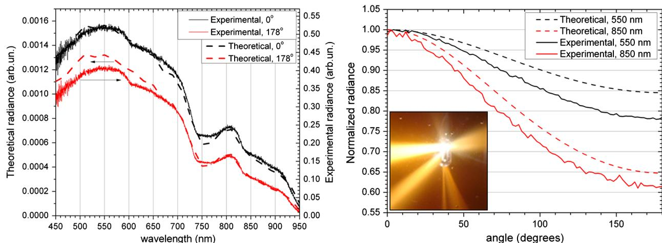
**Fig. 3** (a) Spectral radiance (experimental and theoretical) for Intralipid-1% at 0 deg and 178 deg. (b) Angular radiance (normalized, experimental and theoretical) for Intralipid-1% for 550 nm and 850 nm. Inset: light beams coming from the side firing fiber.
