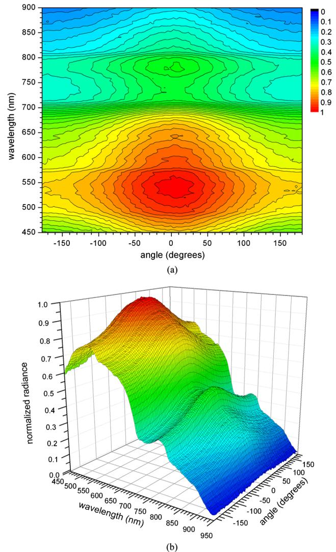
**Fig. 4** (a) Experimental contour plot (normalized) of the spectro-angular distribution of radiance in Intralipid-1%. (b) Experimental surface plot (normalized) of the spectro-angular distribution of radiance in Intralipid-1%. All for 12 mm source-detector separation (the same color coding for both plots).
