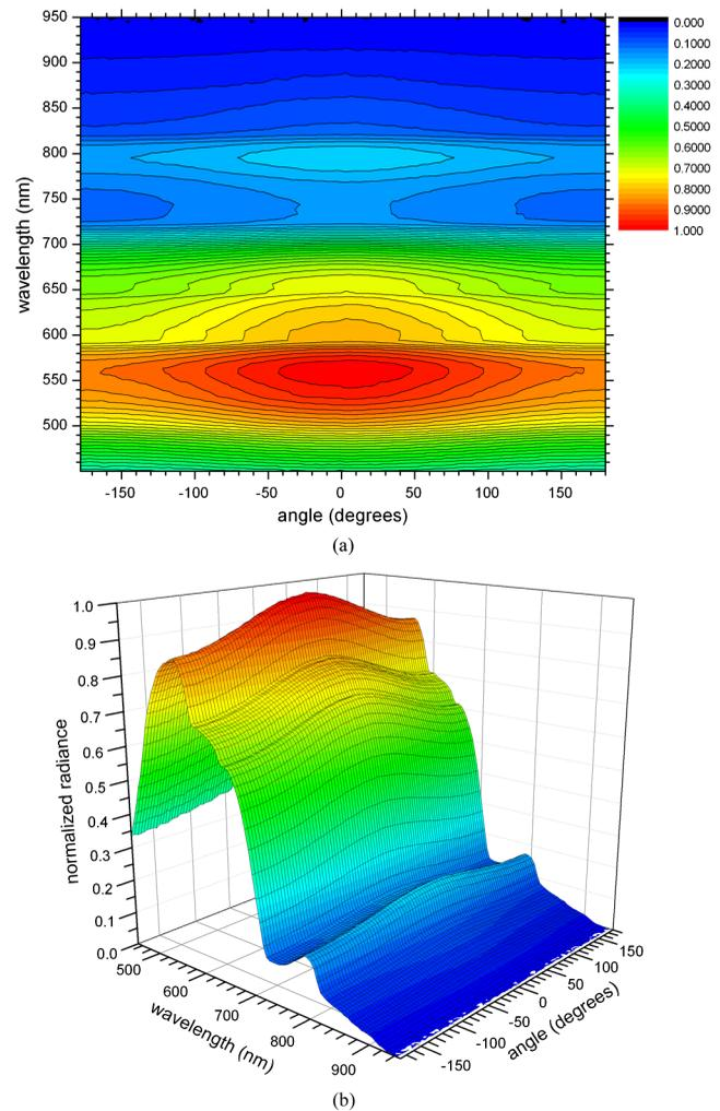
**Fig. 8** Experimental contour plot of the spectro-angular distribution of radiance (a) and experimental surface plot of the spectro-angular distribution of radiance (b) in Intralipid-1% for 30.5 mm source-detector separation (the same color coding for both plots).
