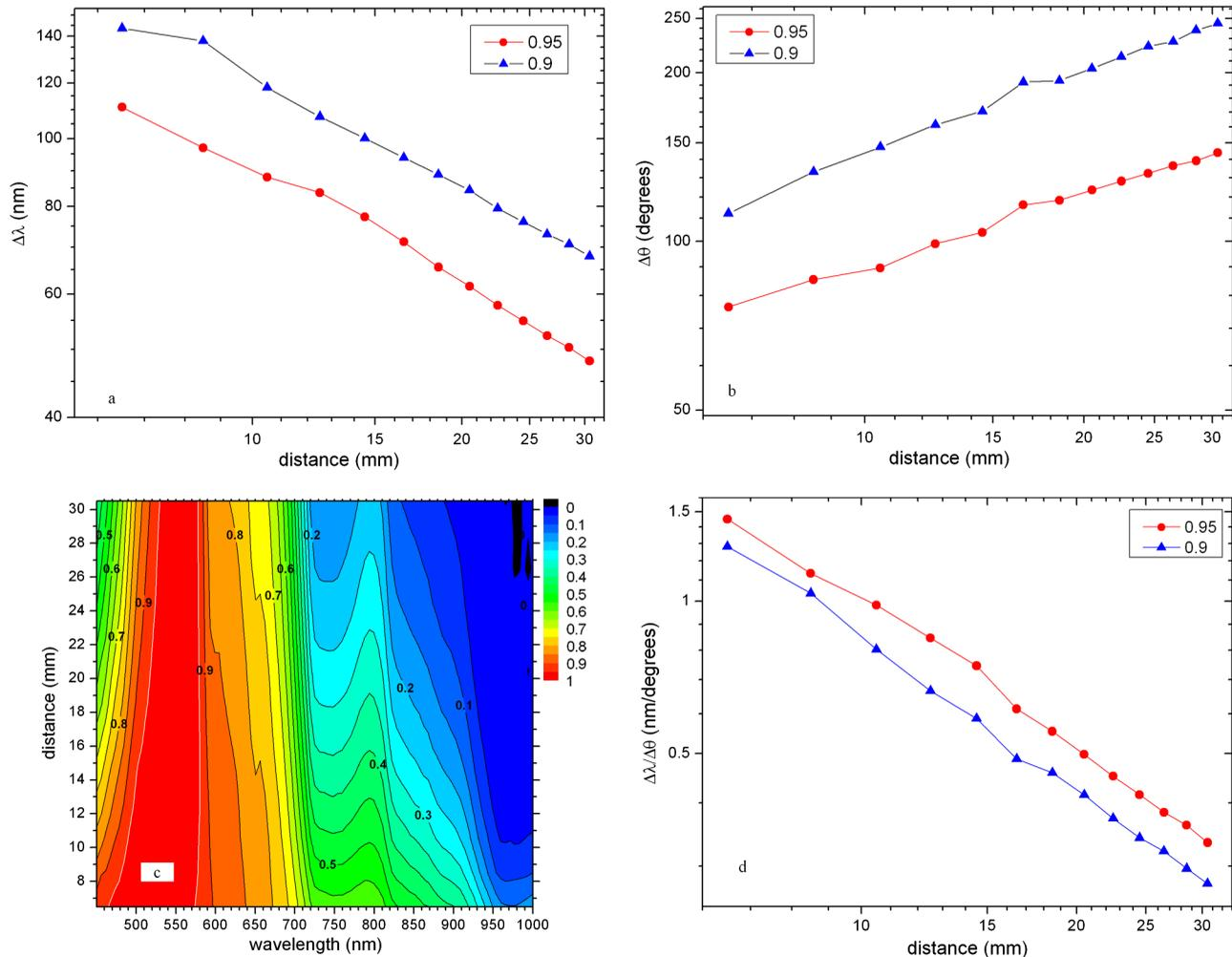
**Fig. 9** Distance dependence for the spectral,  $\Delta\lambda$  (a) and angular,  $\Delta\theta$  (b) ranges produced by contour lines at 0.9 and 0.95 levels of the experimental spectro-angular contour plots. Part (c) shows a spectro-spatial contour plot that correctly predicts  $\Delta\lambda$  (contour line for 0.95 level is in white) Part (d) shows a ratio of  $\Delta\lambda/\Delta\theta$ .
