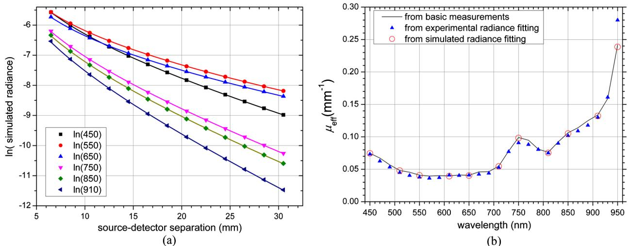
Fig. 6 (a) Simulated distance dependent radiance for selected wavelengths in Intralipid-1%. (b) The effective attenuation coefficient of Intralipid-1%.
