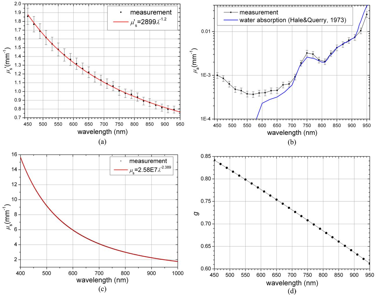
**Fig. 2** Optical parameters of Intralipid-1% from basic characterization measurements: (a) the reduced scattering coefficient,  $\mu'_s(\lambda)$ , (b) the absorption coefficient,  $\mu_a(\lambda)$ , (c) the scattering coefficient,  $\mu_s(\lambda)$ , (d) the anisotropy factor,  $g(\lambda)$ .
