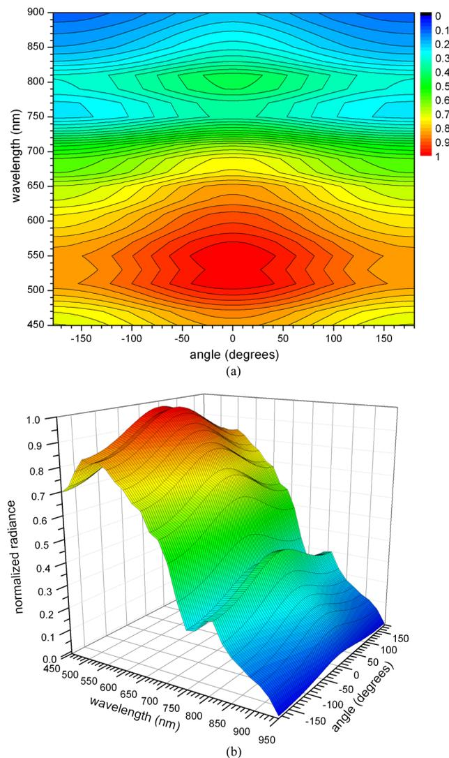
**Fig. 5** (a) Simulated contour plot (normalized) of the spectro-angular distribution of radiance in Intralipid-1%. (b) Simulated surface plot (normalized) of the spectro-angular distribution of radiance in Intralipid-1%. All for 12 mm source-detector separation (the same color coding for both plots).
