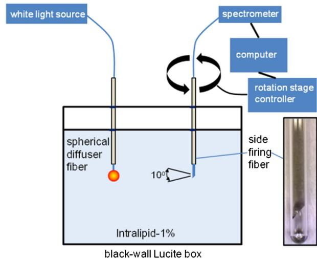
Fig. 1 The schematic of the experimental setup. The inset shows a tip of the side firing fiber.
