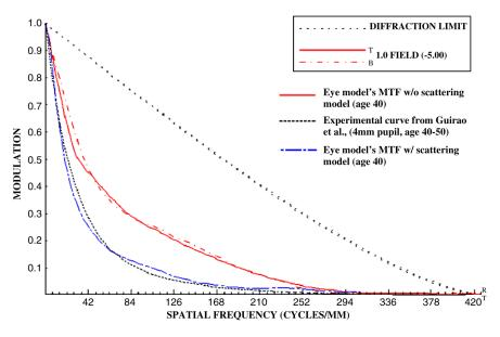
Fig. 6 Monochromatic MTF of the eye model for age 40 at 555 nm wavelength.
