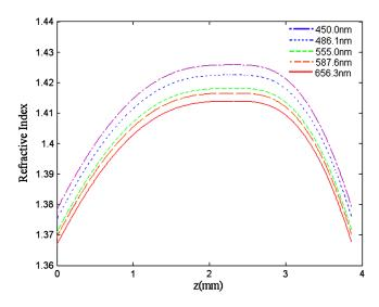
Fig. 8 Refractive-index curves of the crystalline lens along the optical axis at five wavelengths.
