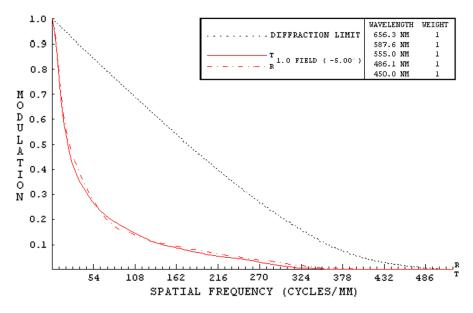
Fig. 10 MTF with five equally-weighted wavelengths at 450.0, 486.1, 555.0, 587.6, and 656.3 nm.
