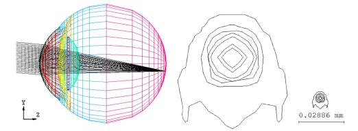
Fig. 5 Schematic of the human eye model in ASAP (left) and the corresponding PSF on the retina for an object at infinity at 555 nm (right). The contours in PSF represent intensity distributions at 75%, 65%, 45%, 35%, 25%, 15%, and 5% of the maximum intensity.
