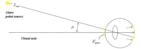
Fig. 4 Illustration for a glare point source at infinity, its irradiance at the cornea, and the veiling luminance of the glare source contributed to the light received at the fovea.
