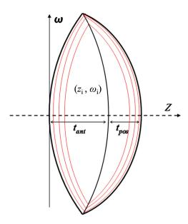
Fig. 3 Illustration of the GRIN lens model with concentric conicoid isoindical surfaces.
