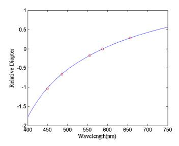
**Fig. 9** Chromatic difference of the optical powers obtained from the eye model at five wavelengths. The blue line represents the human dispersion curve based on experimental data.
