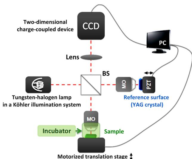
**Fig. 1** Schematic diagram of FF-OCT based on the Linnik interference microscope. BS, beam splitter; MO, microscope objectives (water-immersion, 20×, 0.4 NA); Lens (300 mm focal length); PZT, piezoelectric transducer; CCD, 2-D silicon charged-coupled device; PC, personal computer.
