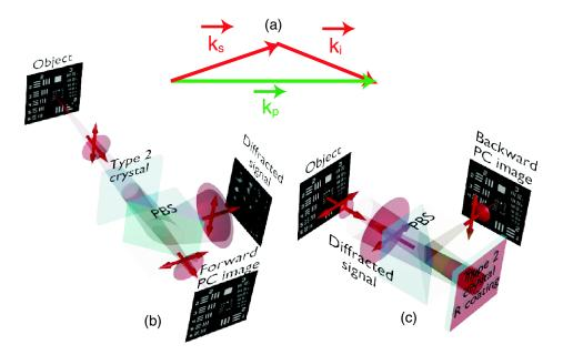
**Fig. 2** (a) k-wavevector diagram for noncolinear three-wave mixing. (b) Principle of forward three-wave mixing phase-conjugation imaging. (c) Full phase-conjugation by three-wave mixing. The horizontal and vertical arrows represent the crossed polarization directions of the signal and idler waves in a type 2 interaction. For the sake of clarity, the pump plane wave is not represented.
