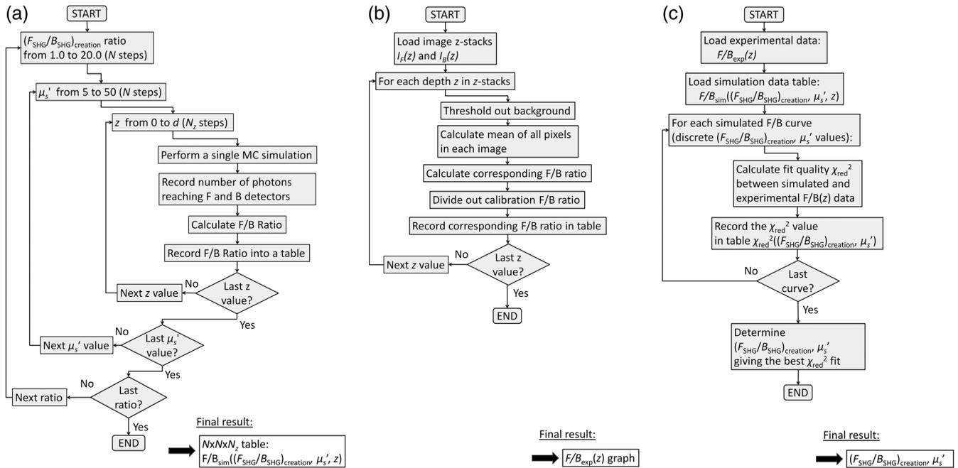
**Fig. 4** Flowcharts illustrating the full process going from data acquisition to obtaining  $(F_{\text{SHG}}/B_{\text{SHG}})_{\text{creation}}$  from fitting to simulations. (a) Generation of forward simulations, (b) loading of experimental data, and (c) fitting experimental to simulated data.
