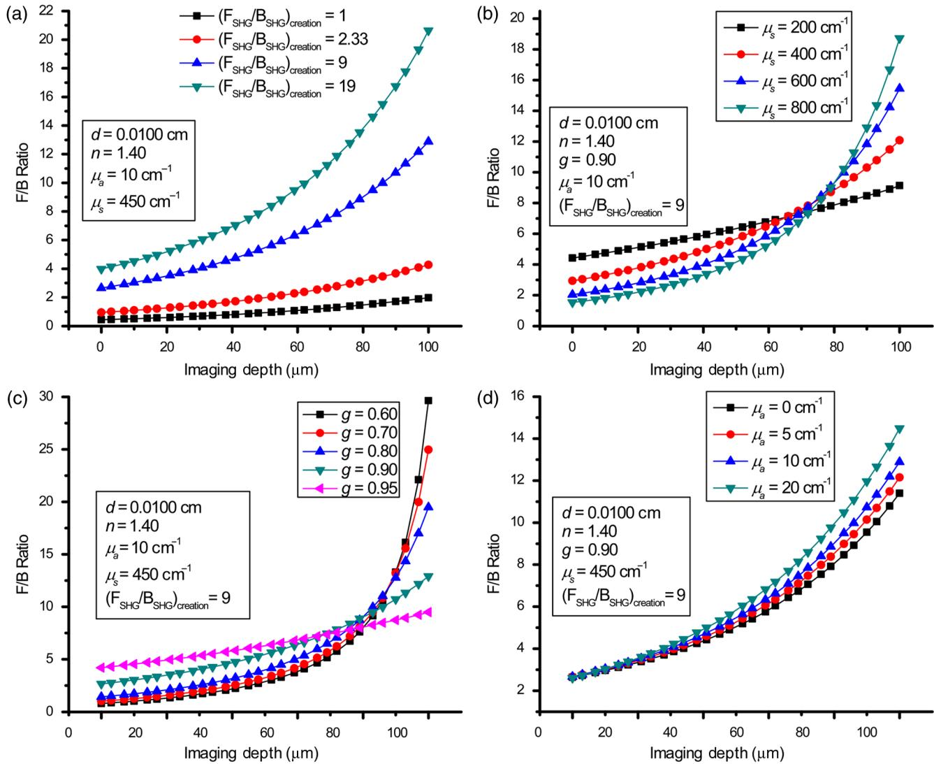
**Fig. 3** Effects of the following optical parameters on the depth-resolved F/B ratio through simulations. (a)  $F_{\text{SHG}}/B_{\text{SHG}}_{\text{creation}}$ ,  $\mu_s$ ,  $g$ , and  $\mu_a$ . Other parameters were kept fixed as indicated in each figure.
