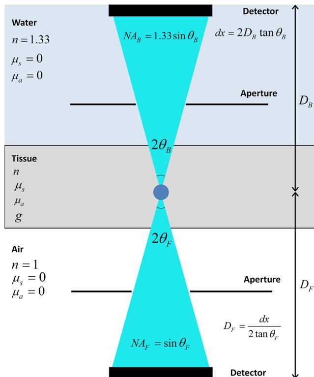
**Fig. 1** Monte Carlo simulation geometry for collection of the second-harmonic generation (SHG) signal, where  $D_B$  and  $D_F$  denote the distances from the focus to the backward and forward detectors, respectively, and  $\theta_F$  and  $\theta_B$  are the collection angles defined by the condenser and objective for forward and backward SHGs, respectively.
