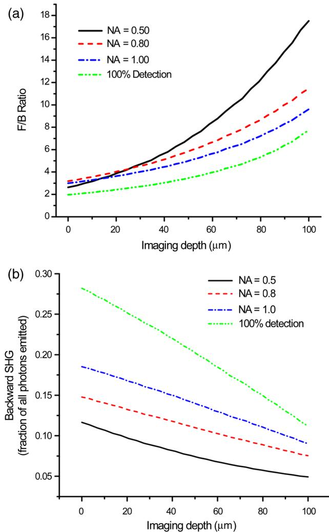
**Fig. 2** Effects of collection aperture with 0.8 numerical aperture excitation on the depth-resolved forward/backward (F/B) (a) and backward SHG responses using previously determined bulk optical property measurements on tendon.
