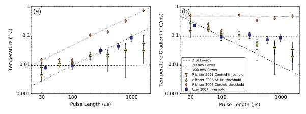
**Fig. 8** (a) Simulated peak temperature changes and (b) average temperature gradient resulting from INS at a wavelength of 1850 nm, for pulse lengths between 10  $\mu$ s and 2000  $\mu$ s. Experimental stimulation thresholds from Izzo et al.<sup>20</sup> and Richter et al.<sup>29</sup> are included for comparison.
