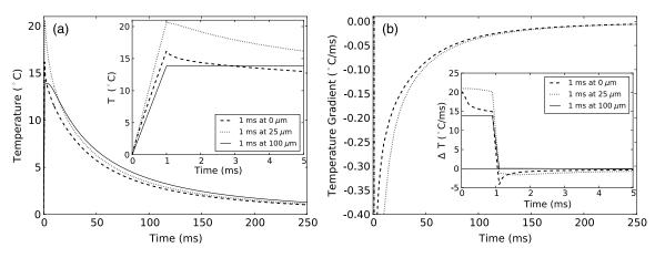
Fig. 5 Change in temperature during INS pulse and the resulting decay using the geometry used by Shapiro et al.6
