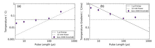
**Fig. 9** (a) Simulated temperature changes and (b) temperature gradient resulting from INS at a wavelength of 1937 nm, for pulse lengths between 10  $\mu$ s and 1000  $\mu$ s. Data from Izzo et al.<sup>17</sup> is included for comparison.
