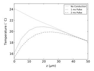
Fig. 4 Change in temperature at end of 1 and 2 ms pulses and with no heat conduction considered.
