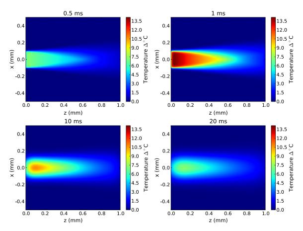
Fig. 3 Change in temperature from a 1 ms pulse ( $E_{pulse} = 2$  mJ) at 0.5, 1, 10, and 20 ms.
