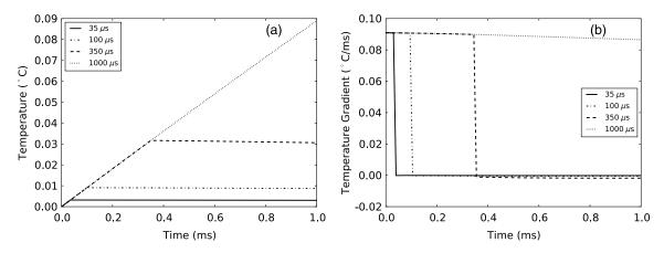
Fig. 7 (a) Change in temperature during 35  $\mu$ s, 100  $\mu$ s, 350  $\mu$ s and 1 ms pulses, all with laser power of 20 mW; (b) temperature gradient during 20 mW pulses.
