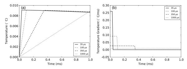
Fig. 6 (a) Change in temperature during 35 μs, 100 μs, 350 μs and 1 ms pulses, all with an energy of 2 μJ; (b) temperature gradient during 2 μJ pulses.
