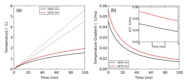
Fig. 1 (a) Temperature rise generated by a 10 mW laser running CW over 100 ms: solid lines show the temperature with conduction taken into account; dashed lines show the temperature if there was no conduction; (b) temperature gradient from a 10 mW laser running CW over 100 ms.
