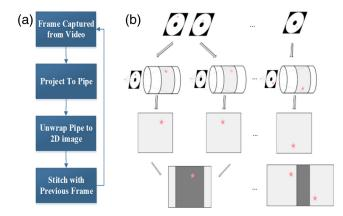
**Fig. 3** (a) A flowchart shows the pipeline of image stitching software. (b) Graphical illustration of the pipeline.
