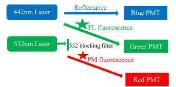
**Fig. 4** Dual-mode fluorescence-reflectance two-fluorophore imaging. The 632-nm laser is powered off. The 532-nm laser is blocked in front of the green detection channel, only allowing fluorescence signal to pass through. Therefore, the green and red detection channels are configured for fluorescence imaging, whereas the blue detection channel is for reflectance imaging.
