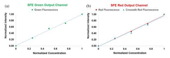
**Fig. 8** Fluorescence dye-in-polymer concentrations were plotted against the detected fluorescence signals in the SFE images. Specifically, (a) shows the dependence for the SFE green detection channel and (b) shows the dependence for the SFE red detection channel. The data shows that a linear relationship exists for both (a) and (b) cases.
