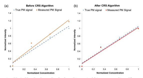
**Fig. 12** Comparison of the signal from the red output channel to the true PM targets signal during concurrent multispectral fluorescence imaging. (a) Before applying the CRS algorithm, the red fluorescence signal from the red detection channel (solid line) deviated from the true PM curve (dashed line). (b) After applying the CRS algorithm, the red fluorescence signal (solid line) closely matched the true PM fluorescence curve (dashed line).
