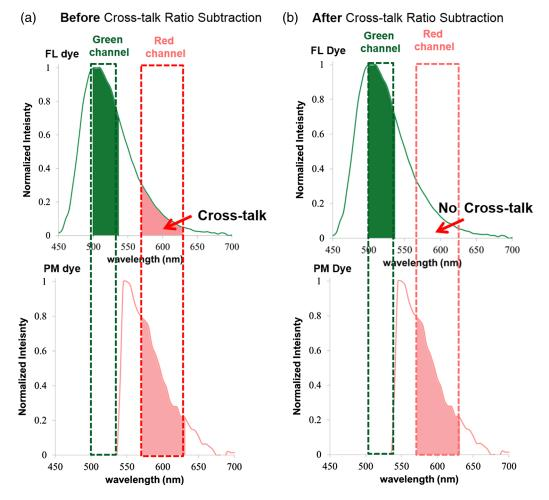
**Fig. 9** Graphic illustration of concurrent multispectral imaging before (a) and after (b) applying the CRS method. (a) Before the CRS algorithm, PM dye signal and a confounding FL dye cross-talk signal were detected in the concurrent red channel. (b) After the CRS algorithm, the FL cross-talk was mitigated and only the true PM dye signal was detected in the red channel.
