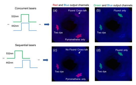
Fig. 13 Concurrent laser excitation compared with sequential laser excitation results. In concurrent laser excitation, the FL cross-talk signal was observed in the red output channel in (a), whereas in sequential laser excitation, only PM fluorescence signal was received in the red output channel, and no FL cross-talk was observed (c). The green output channel remained the same under both concurrent (b) and sequential (d) laser excitation, as there was no cross-talk in the green output channel.
