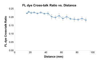
**Fig. 10** The FL cross-talk ratio was plotted as a function of the distance between the distal end of the SFE endoscope and the fluorescence target. The ratio remained constant ( $0.225 \pm 0.012$ ) over a distance range of 15 to 40 mm and remained relatively consistent ( $0.207 \pm 0.025$ ) across a distance of 15 to 95 mm.
