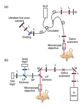
**Fig. 1** Systematic diagram of (a) OMAG and (b) MPM imaging systems. L: lens; M: mirror; SLD: superluminescent laser diode; LP Dichroic: long-pass dichroic beamsplitter.
