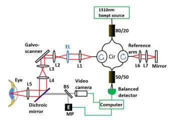
**Fig. 1** Schematics of dynamic-focusing swept-source optical coherence tomography (SS-OCT) system. Cir, circulator; MP, miniprojector; EL, electrical lens; and L1–L7 as the lens number from 1 to 7.
