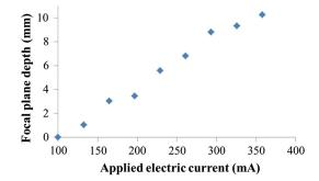
Fig. 3 Relationship between focal plane depth and current applied to the electrical lens.
