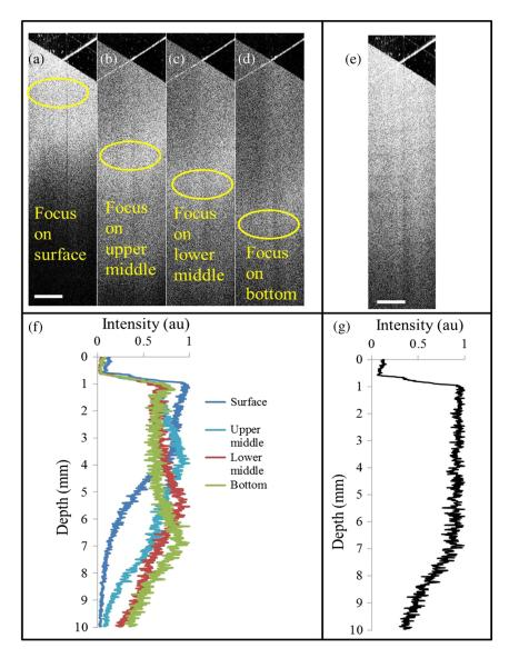
**Fig. 2** SS-OCT images of 0.1% intralipid solution obtained at different focal depths. (a)–(d) Images obtained with focal planes at the surface, upper middle, lower middle, and bottom region of intralipid solution. (e) The composite image generated by fusing the Gauassian-weighted window filtering of images (a)–(d). (f) The axial intensity profile for images in (a)–(d). (g) The axial intensity profile for the composite image in (e).
