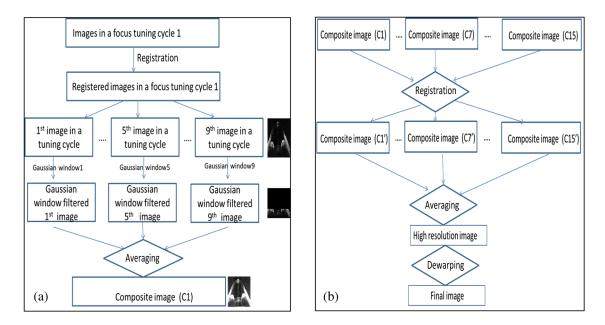
**Fig. 5** Flowchart of dynamic-focusing OCT image process. (a) Procedure to get the composite image from the images in a focus tuning cycle. (b) The procedure in (a) is repeated for different tuning cycles to get different composite images. The composite images are further registered and averaged to get a high-resolution image with reduced speckles. The high-resolution image was dewarped to get the final image.
