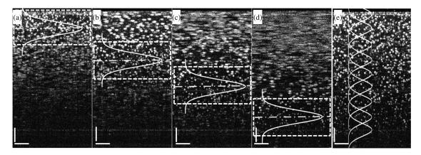
**Fig. 4** Imaging microbeads by dynamic-focusing SS-OCT system. (a)–(d) The images of microbeads obtained when the focal planes were set from the surface to the bottom of the cuvette. (e) The composite image by averaging the Gaussian-filtered image frames. Microbeads diameter: 9.6  $\mu$ m. The scale bars are 1 mm.
