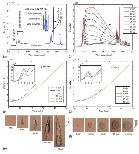
**Fig. 3** Liquid samples were illuminated with a 600  $\mu$ m fiber. (a) Background signal recorded when immersing the probe into water. (b) Spectra over time during photopolymerization of a poly(ethylene glycol) dimethacrylate (PEGDMA) sample. (c) The change in intensity over time for different samples measured at 580 nm without nano-fibrillated cellulose (NFC) fibers and (d) with NFC fibers. (e) Resulting volumes after photopolymerization without NFC fibers and (f) with NFC fibers
