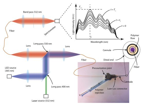
**Fig. 2** Schematic illustration of the illumination and detection system. The sample is illuminated with a light-emitting diode light source (365 nm) to photopolymerize the injected photoreactive precursor and with a green light source (532 nm) to monitor photopolymerization. The spectrometer records the back-scattered fluorescence and Raman spectra. The distal tip of the device consists of a cannula containing the optical fiber and a circular chamber to inject the liquid photopolymer.
