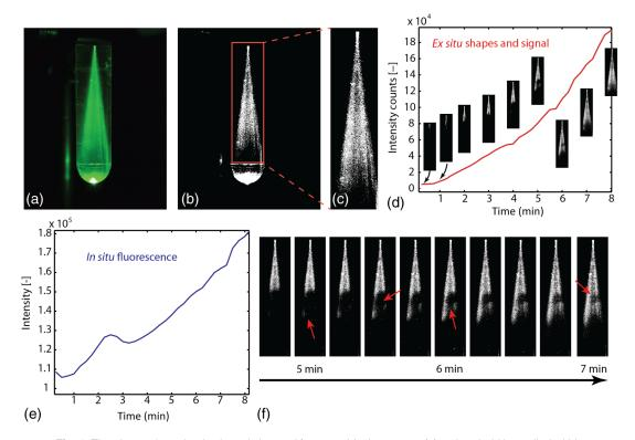
**Fig. 4** The photopolymerized volume is imaged from outside the cuvette (a), a threshold is applied within a relevant area (b) and (c) and by a pixel count the size and the signal intensity plotted over time (d). The *ex situ* signal does not show any peak between 2 and 4 min, while during *in situ* monitoring of the same sample such a peak appears (e). Detail of the evolution of the sample size and geometry over time (f).
