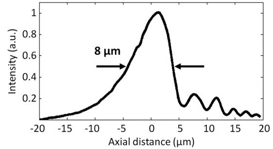
**Fig. 3** Measured axial response of the SESCOm-SS setup.
