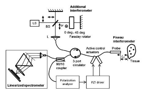
**Fig. 1** CP OCT schematic. LS, light source; BS, beam splitter; L, lens; and  $L_0$ , interferometer offset. Reprinted, with permission, from Gubarkova et al.<sup>11</sup>
