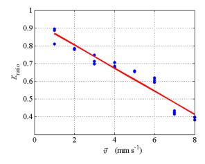
**Fig. 4** Relationship between speckle contrast and the velocity of the moving fluid. The fluid phantom had a reduced scattering coefficient of 2.2 mms<sup>-1</sup>. The correlation coefficient,  $r^2 = 0.96$ .
