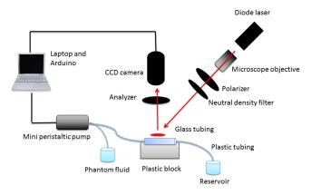
Fig. 1 Diagram of the LSCI and flow systems.
