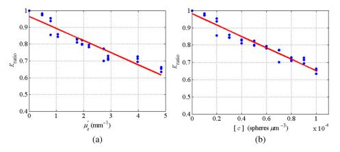
**Fig. 3** (a)  $K_{\text{ratio}}$  versus reduced scattering coefficient. A strong negative correlation ( $r^2 = 0.95$ ) was found between the two variables. The slope of the best-fit line was -0.072. (b)  $K_{\text{ratio}}$  versus scatterer concentration. A strong negative correlation ( $r^2 = 0.97$ ) was found between the two variables. The slope of the best-fit line was  $-3.3 \times 10^{-3}$ .
