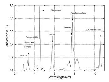
**Fig. 2** Absorption spectra of gas mixture in the reference cell in the spectral range from 2500 to 10,700 nm.
