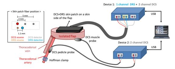
**Fig. 2** Two identical perfusion-monitoring devices (controlled by custom software in one laptop via USB) have been set up for multisite flap monitoring through different types of optical probes: skin patch, pedicle, and muscle probe. The inset diagram displays probe geometry for DCS and DRS in the skin optical patch.
