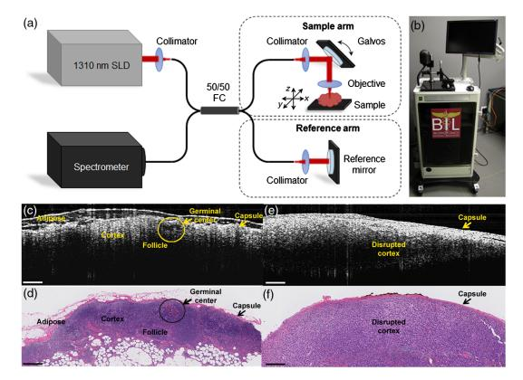
**Fig. 3** Second-generation intraoperative portable spectral-domain OCT clinical system. (a) OCT system schematic and (b) photo of the OCT system. Physical dimensions were greatly reduced over the previous version. (c, e) Representative intraoperative OCT and (d, f) corresponding histopathology images of a normal, nonmetastatic (left) and cancerous metastatic (right) *ex vivo* human LNs. All scale bars represent 0.5 mm. Modified and reprinted with permission.<sup>53</sup>
