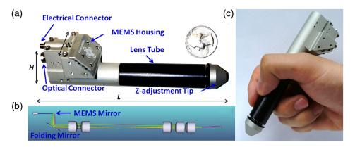
**Fig. 23** Intraoperative MEMS-based handheld Doppler OCT probe to observe microvascular anastomosis. (a) CAD design of handheld probe compared to US currency (quarter). (b) Interior optical design within probe. (c) Handheld probe in hand. Reprinted with permission. <sup>168</sup>
