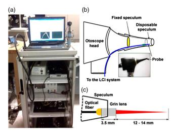
**Fig. 5** (a) Portable LCI-otoscopy system. (b) Schematic and photograph of the integration of the LCI fiber-based micro-optic probe into an ear speculum tip that would attach to the otoscope head. (c) Schematic and beam profile of the long-working-distance LCI probe, which used a gradient-index (GRIN) lens. Modified and reprinted with permission. <sup>71</sup>
