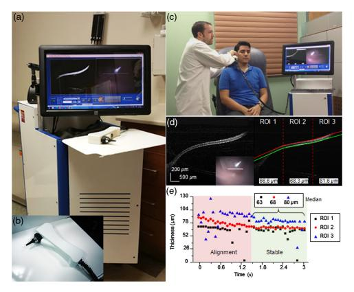
**Fig. 8** Second-generation primary care system and handheld probe. (a, b) Portable system and handheld probe in the primary care clinic. (c) System in use within our clinical imaging suite. (d) Automated segmentation and thickness analysis of an *in vivo* human TM. (e) Real-time thickness measurement tracking over time. Modified and reprinted with permission.<sup>80,81</sup>
