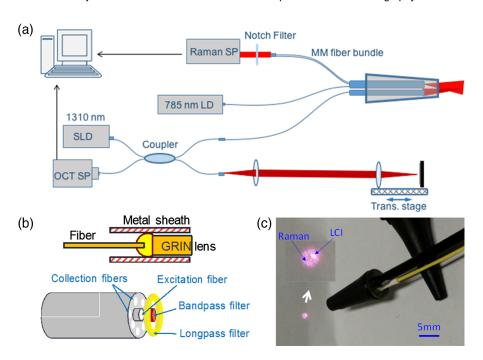
**Fig. 24** Multimodal handheld probe for sampling ear infections. (a) Schematic setup of the multimodal RS-LCI probe. (b) Schematic of the LCI (top) and RS (bottom) components. (c) Photograph of the fiber-based RS-LCI probe encapsulated into an ear speculum. The inset shows magnified view of both the RS and LCI beam. Abbreviations: SP, spectrometer; LD, laser diode; SLD, superluminescent diode; and MM, multimode. Reprinted with permission.<sup>178</sup>
