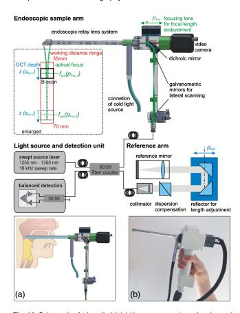
**Fig. 18** Schematic of a handheld rigid laryngoscope-based probe and OCT system. The working distance of the OCT-laryngoscope optical focus can be adjusted by the automated focusing lens, indicated in green, and by the OCT reference arm path-length, indicated in blue. (a) Handheld probe and interrogation area near vocal folds. (b) Photo of handheld probe. Reprinted with permission. <sup>126</sup>
