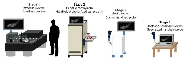
**Fig. 1** Visual representation of stages 1 to 4 OCT systems. As system form factor is reduced, tradeoffs between image quality (SNR, phase stability, resolution, weight, and scan speed) and portability must be managed. For later-stage systems, reducing cost becomes more of a concern as well. Eventually, image quality and system capabilities become more focused on meeting the needs of a clinical application or a commercial product at a specific price point.
