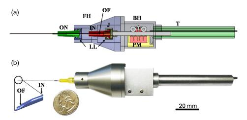
**Fig. 22** SMART handheld. (a) CAD design cross section. Abbreviations: FH, front holder; BH, back holder; J, joint; T, tail; ON, outer needle; IN, inner needle; PM, piezoelectric motor; LL, luer-lock combination; OF, optical fiber. (b) Completed probe, compared to a quarter (US currency). Reprinted with permission. <sup>167</sup>
