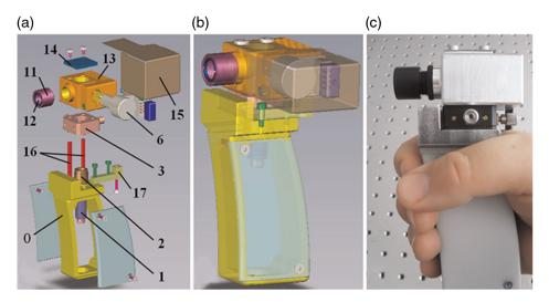
**Fig. 21** Handheld OCT scanner with a one-dimensional galvanometer-based scanner, suitable for small-scale production. (a, b) Exploded view (itemized) and transparent CAD design of the assembly. 17–1: optical components (see citation). (c) Completed handheld probe. Reprinted with permission. <sup>154</sup>
