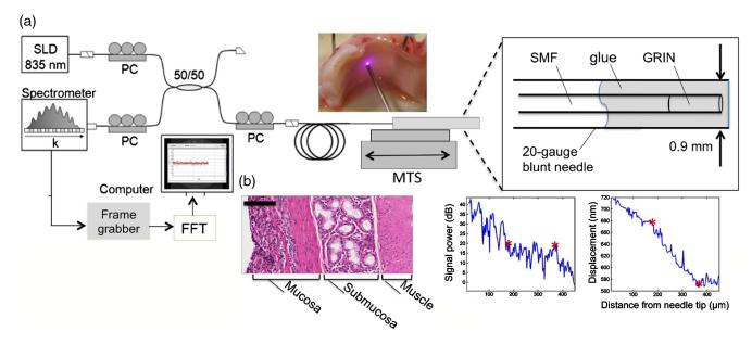
**Fig. 20** Tissue boundary detection using OCT-elastography in a handheld needle probe. (a) Schematic of forward facing needle probe and OCT system. Abbreviations: SLD, superluminescent diode; PC, polarization controller; MTS, motorized translation stage; SMF, single-mode fiber; GRIN, gradient-index fiber. (b) Boundary detection in *ex vivo* porcine tracheal wall with comparative histology. Scale bar represents 100  $\mu$ m. Reprinted with permission.<sup>138</sup>
