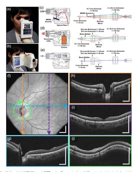
**Fig. 14** Handheld MEMS-based OCT probe. Demonstration of different grip styles including (a) "power grip" and (b) "camcorder" styles. (c–e) Optical layouts of (c) OCT 1060 nm optical path, (d) iris camera visible optical path, and (e) fixation target visible optical path. (f–j) Motion-corrected widefield volume; (f) *en face* OCT fundus image. (g–j) Color-indicated OCT scans from various regions in the retina. Modified and reprinted with permission. <sup>111</sup>
