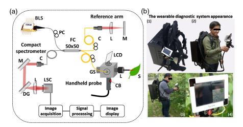
**Fig. 28** Backpack OCT system for crop QC. (a) Schematic of the portable, compact, and battery-powered backpack-OCT system. (b) (1) wearable system, (2) user wearing pack, (3) user scanning plant leaves, and (4) handheld LCD screen. Reprinted with permission. <sup>187</sup>
