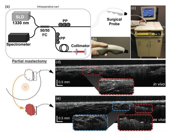
**Fig. 4** Third-generation intraoperative portable OCT system and handheld probe. (a) System schematic and (b) handheld probe, when used with surgical sheath, can be used intraoperatively and *in situ*. (c) Handheld probe and OCT system in portable cart. (d) *In vivo* images from a partial mastectomy margin. (e) *Ex vivo* confirmation of conjugate side. OCT images were correlated and confirmed with corresponding histology. Reprinted with permission.<sup>56</sup>
