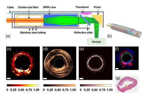
**Fig. 27** Integrated multimodal (OCT, US, and PAI) probe. (a) Schematic of distal end of probe and optical path. (b) CAD rendering of the probe. (Bottom) Cross-sectional images of human artery with atherosclerotic plaque. (c) PAI image, (d) US image, (e) OCT image, (f) color-coded RGB image, and (g) H & E histology. Reprinted (adapted) with permission from Ref. 186. Copyright (2016) American Chemical Society.
