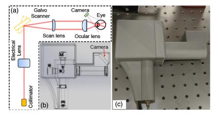
**Fig. 15** Handheld OCT angiography probe with automated tunable lens focus adjustment. (a) Schematic of the handheld OCTA probe. (b) 3-D perspective view of the probe including all the optical components and the designed plastic case for mounting and holding. (c) Photograph of the handheld OCTA probe with 3-D-printed enclosure. Reprinted with permission. <sup>114</sup>
