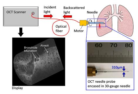
**Fig. 19** Schematic of a handheld OCT needle probe system with a 30-gauge needle. Display shows the 3-D visualization of a fetile lamb lung showing alveoli and bronchiole bifurcations. Length of cylindrical scan is 2 mm. Reprinted with permission.<sup>132</sup>
