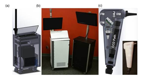
**Fig. 10** Third-generation primary care imaging portable system and handheld probe. (a) CAD schematic of cart layout and interior organization. (b) Portable systems testing different material choices (left: powder-coated metal frame and side panels; right: aluminum frame and plastic panels). (c) Schematic of handheld probe layout and final 3-D-printed enclosure. FM, fold mirror; CO, collimation optics; OBJ, objective lens; DM, dichroic mirror.
