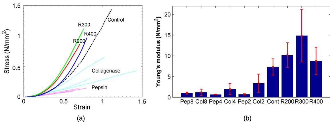
**Fig. 3** (a) Mean stress–strain curves, obtained by averaging the stress–strain curves of each experimental group. (b) Mean YM for all experimental groups, with their corresponding standard deviation.
