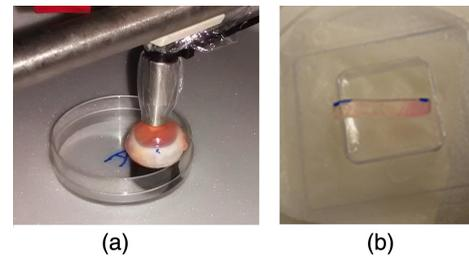
**Fig. 1** (a) Fluorometer probe placed atop the rabbit eye. The probe was covered with a plastic film to avoid contamination. (b) Corneal strip excised after staining and irradiating the eye.
