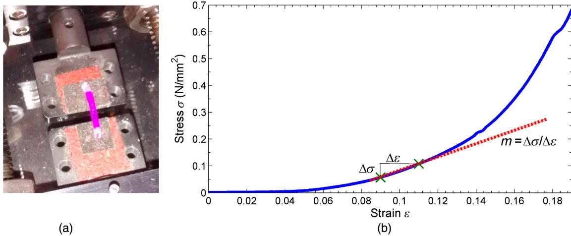
**Fig. 2** (a) Corneal strip on grips of tensiometer. (b) Typical stress–strain curve produced by the tensiometer. Two points on the curve were selected around a 10% extension of the original length (0.1 strain) and the YM was calculated as the slope between them.
