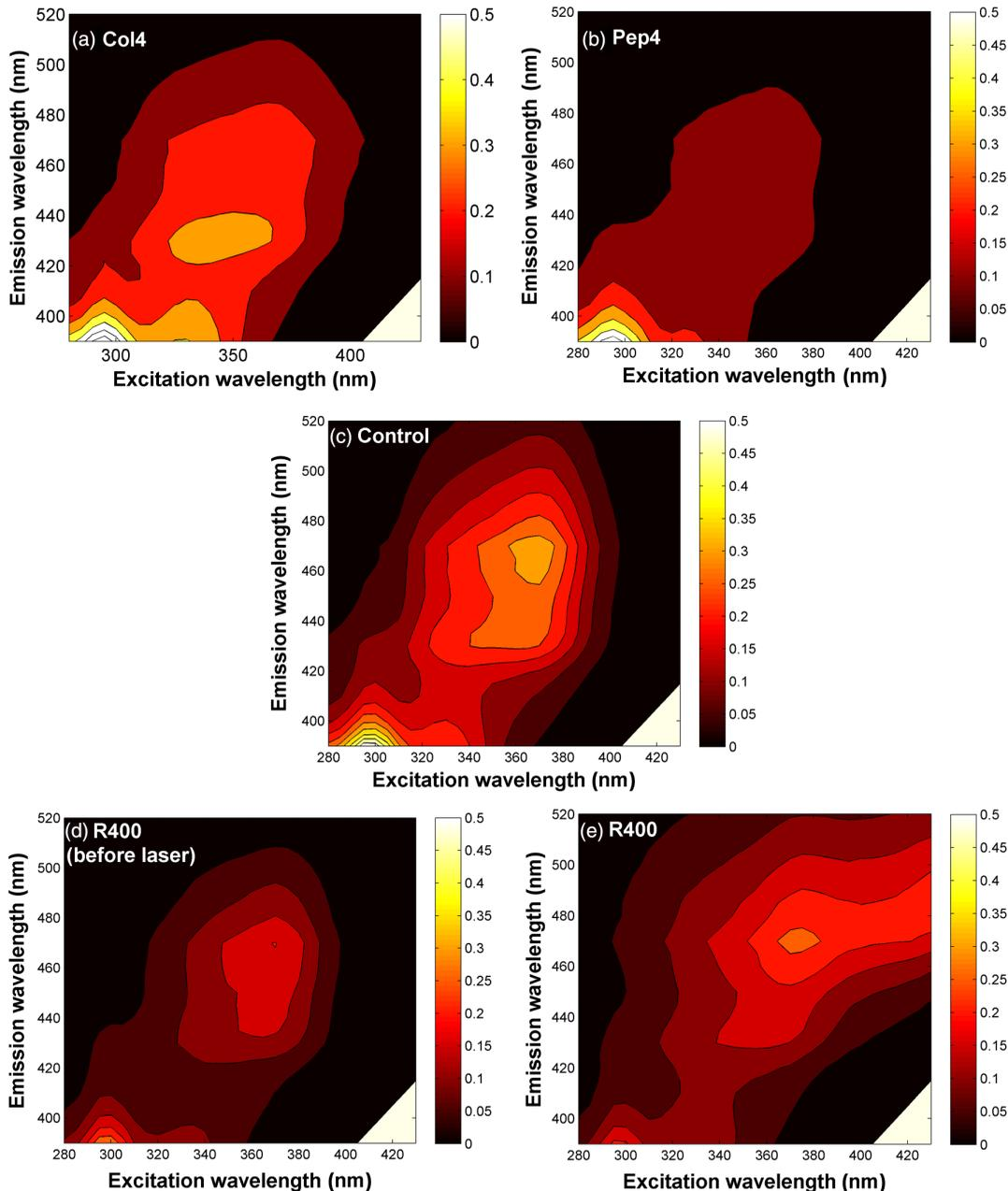
**Fig. 4** Average EEMs for five representative cases of the experimental groups: (a) collagenase-treated samples, 4 h; (b) pepsin-treated samples, 4 h; (c) control untreated samples; corneas after staining with rose bengal, (d) before irradiation, and (e) after 400 J/cm<sup>2</sup> irradiation with green laser light.
