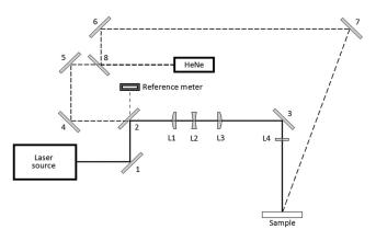
**Fig. 1** Optics diagram, (1–3) high-reflectivity mirrors for 1070 nm; (4–7) silver mirrors; (8) 50/50 beam splitter; (L1) positive lens; (L2) negative lens; (L3) positive lens; (L4) planoconvex lens for changing between 3- and 7-mm diameters. The small amount of transmitted light through (2) is captured by a reference meter.
