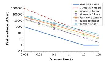
**Fig. 9** MPE defined by ANSI Z136.1-2014,<sup>45</sup> ablation onset threshold calculated by the 1-D ablation model,<sup>12</sup> MVL thresholds from Vincelette et al.<sup>3</sup> for 6- and 11-mm beam diameters, and progressive damage thresholds from this experiment.
