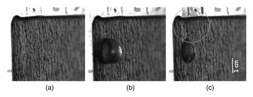
Fig. 5 Bubble rupture injury event (a) pre-exposure, (b) intraexposure, and (c) at point of rupture, with the circle showing steam and material ejecting from the blister.
