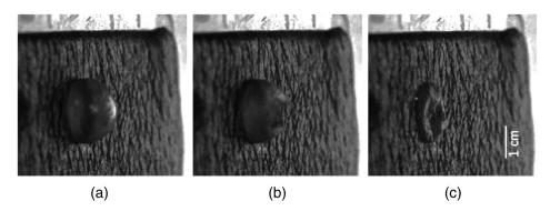
Fig. 6 Bubble rupture injury event with a "tensile limit" rupture (a) intraexposure, (b) at point of rupture, and (c) postrupture bubble deflation.
