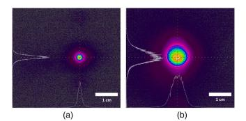
Fig. 2 Beam profiles, experiment II (a) 3-mm diameter and (b) 7-mm diameter.
