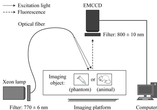
**Fig. 1** A schematic of the fluorescence molecular imaging system. The excitation light from the xeon lamp is filtered through a  $770 \pm 6$  nm filter, and the emitted fluorescence from the imaging object (phantom or animal) is filtered through an  $800 \pm 10$  nm filter before reaching the EMCCD.
