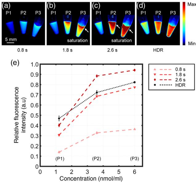
**Fig. 3** (a)–(c) Original fluorescence images of three phantoms (labeled as P1, P2, and P3) filled with 1.2, 3.6, and 6.0 nmol/ml EGF-IRDye probe, with the exposure times of 0.8, 1.8, and 2.6 s, respectively. Saturation areas are indicated by white arrows. (d) HDR result of the phantoms. (e) Relative fluorescence intensity values of phantoms of different concentrations. The error bars indicate the standard deviations of the results from three experiments.
