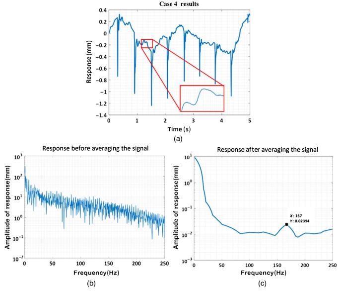
**Fig. 9** (a) Response of the skin in the time domain, (b) response of the skin in the frequency domain extracted using original data case 4, and (c) response of skin in frequency domain extracted after averaging the signal in the frequency domain for test case 4.
