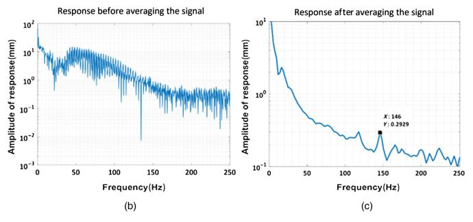
**Fig. 8** (a) Response of the skin in the time domain, (b) response of the skin in the frequency domain extracted using original data case 3, and (c) response of skin in frequency domain extracted after averaging the signal in the frequency domain for test case 3.
