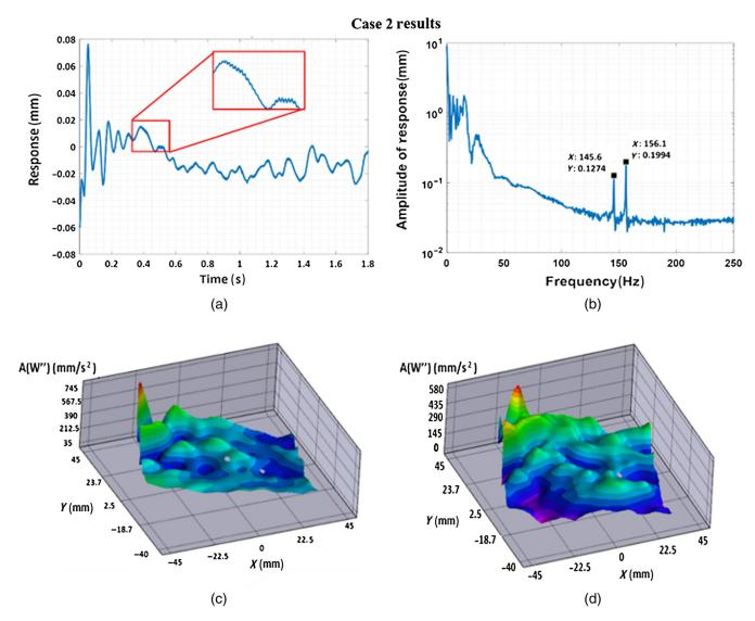
**Fig. 7** (a) Response of the skin in the time domain extracted from MATLAB, (b) response of the skin at 145.6 and 156.1 Hz in the frequency domain extracted from MATLAB, (c) ODSs at 145.6 Hz extracted from DIC measurement, and (d) ODSs at 156.1 Hz extracted from DIC measurement for test case 2.
