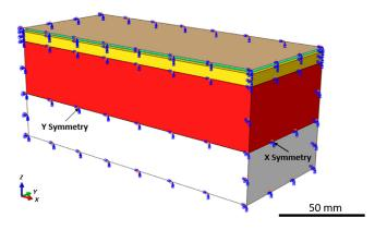
Fig. 2 Symmetric boundary conditions applied on the FE model.
