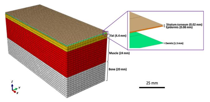
**Fig. 1** The FE model of the human forearm with different layers of skin connected to muscle and bone. The thickness of each layer is obtained from Ref. 38.
