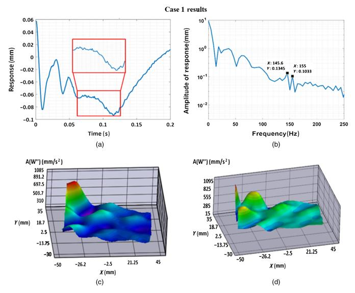
**Fig. 6** (a) Response of the skin in the time domain extracted from MATLAB, (b) response of the skin at 145.6 Hz in the frequency domain extracted from MATLAB, (c) ODSs at 145.6 Hz extracted from DIC measurement, and (d) ODSs at 155 Hz extracted from DIC measurement for test case 1.
