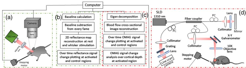
**Fig. 1** Schematic diagram of IOSI and OCT systems and data processing. (a) IOSI system setup, (b) IOSI data processing steps, (c) OMAG data processing steps, and (d) OCT system setup. SLD, superluminescent diode; PC, polarization controller.
