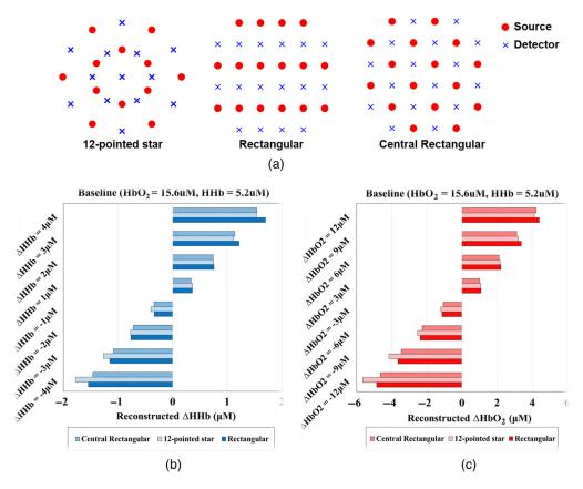
**Fig. 1** (a) Simulated optode topologies. Tomographic reconstruction results for (b)  $\Delta$ HHb and (c)  $\Delta$ HbO<sub>2</sub> from various simulated chromophore perturbations in an embedded inclusion (tumor). Simulation ground truth is indicated on the *y*-axis and reconstructed values are indicated on the *x*-axis.
