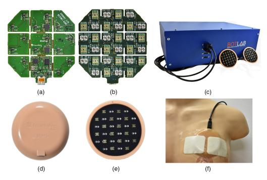
**Fig. 2** (a) Bottom and (b) top copper layers of rigid-flex PCB, as well as (c) back and (d) tissue-facing sides of encased probe. The dimensions of the bare PCB are  $\sim$ 6 cm  $\times$  6 cm, and the encased probe is 8 cm in diameter and 1 cm thick. (e) The peripheral control box with two probes connected via HDMI cable. The dimensions of the box are 42.9 cm  $\times$  32.5 cm  $\times$  14.5 cm. (f) The wearable probe attached to the curved surface of human bust model.
