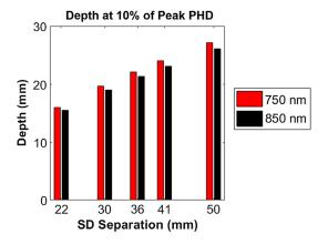
Fig. 6 Depth at 10% of peak photon-hitting density, grouped by wavelength and S-D separation.
