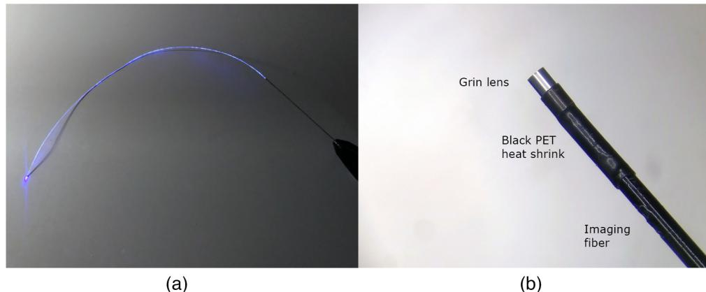
**Fig. 9** (a) Light leaks out of the thin cladding bare fiber and into fluorescent PEEK MLE. (b) Our solution was to replace the clear heat shrink covering the OD of the GRIN lens with black heat shrink.
