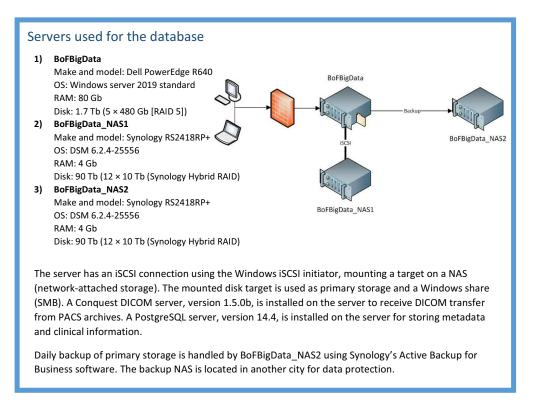
**Fig. 2** Hardware and software of the database's servers with a schematic illustration of its structure and connections. RAID, redundant array of independent disks.
