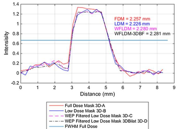
**Fig. 22** Slice containing in-plane vessel, showing profile line (red, blue, magenta, black) used for vessel width measurement. Red FDM (full-dose mask) is scenario A, LDM (low-dose mask) is scenario B, WFLDM-3DBF (WEP filtered 2D, 3D bilateral filtered) is scenario C, and WFLDM (WEP-filtered low-dose mask) is scenario D.
