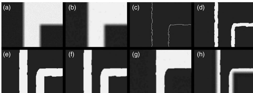
**Fig. 2** WEP filtration stages: (a) input image w/noise  $I_{IN}$ , (b) bilateral-filtered input  $I_{BF}$ , (c)  $I_{Edge}$  is the Canny edges of  $I_{BF}$ , (d) spatial Gaussian dilation  $I_{EdgeDilate}$ , (e) dilation by smoothing filter  $I_{EdgeMask}$ , (f) weighting image  $I_{EdgeWeight}$ , (g) bilateral-filtered part of the WEP composite, and (h) input image edge weighted part of the WEP composite. G and H are added to create  $I_{WEP}$ .
