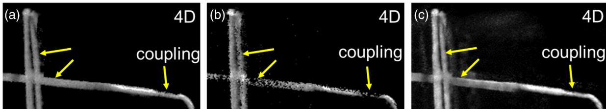
**Fig. 20** ROI in 4D DSA MIPs at frame 133 (sagittal from patient left) using: (a) 100%-dose mask and 100%-dose fill, (b) unfiltered 22.2%-dose mask and 100%-dose fill showing thresholding artifacts, and (c) WEP-filtered 22.2%-dose mask and 100%-dose fill, 3D bilateral filtered.
