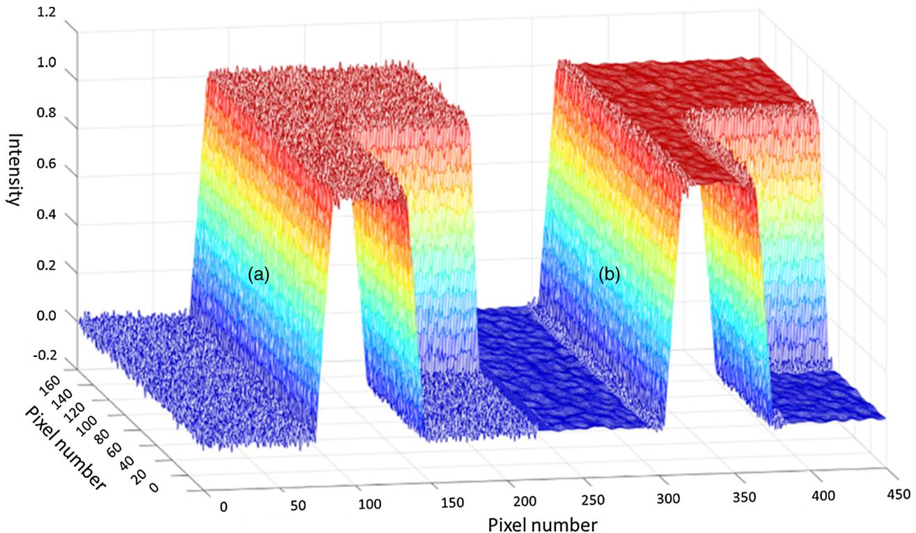
**Fig. 3** (a) Mesh plot of input image [Fig. 2(a)] showing noise texture on the edges and surfaces and (b) mesh plot of WEP filter output [Fig. 2(h)] showing smoothed surfaces outside of the edge regions.
