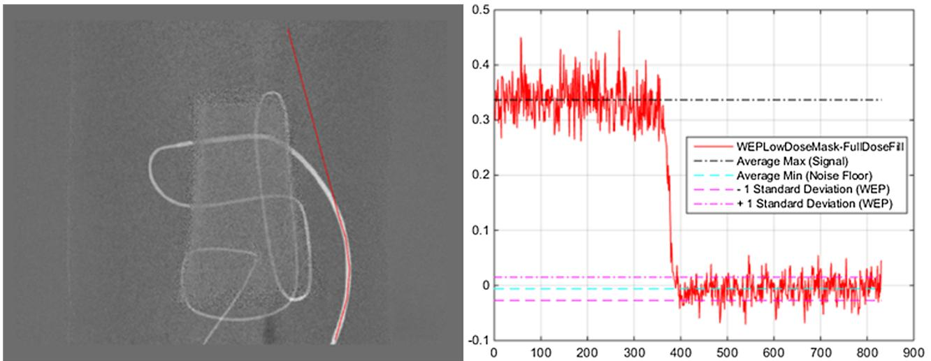
**Fig. 17** Image profile with background and vessel signal used to measure 2D DSA SNR.
