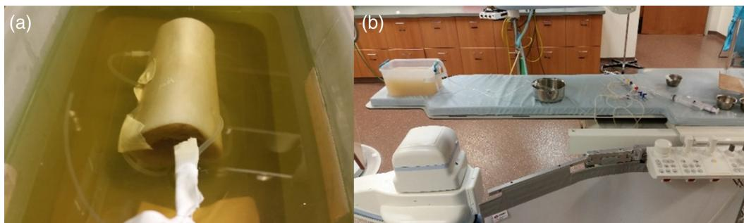
**Fig. 4** (a) Bovine femur-based vascular phantom in agar (unsolidified) and (b) experimental setup.
