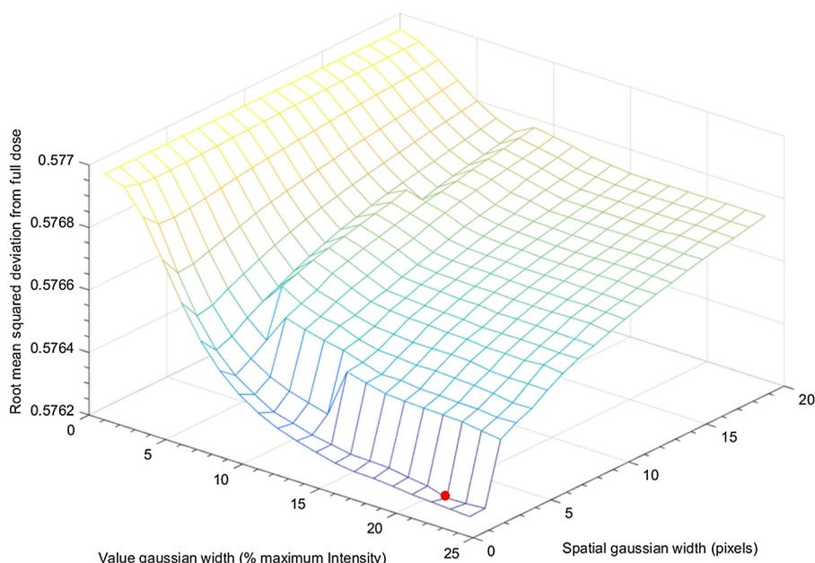
**Fig. 7** Mesh plot of RMSD from full dose to the WEP-filtered low-dose over filter parameter space.
