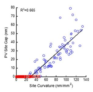
**Fig. 8** Correlation between the remaining gap at each site (see Fig. 7) and the curvature for the corresponding site at a clamping pressure of 80 kPa. Sites that have a gap less than 2 nm (shown in red in the plots) are not included in the correlation as they are considered to be fully chucked.
