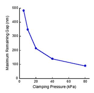
Fig. 6 Maximum remaining gap as a function of clamping pressure for wafer 1. The gap decreases with increasing clamping pressure, but the wafer fails to chuck completely, even at 80 kPa.
