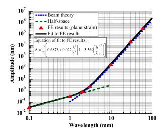
Fig. 2 Maximum amplitude that can be chucked as a function of spatial wavelength. Results from the analytical models and 2-D finite element simulations are shown. A fit to the finite element (FE) results is included to facilitate use of the results.
