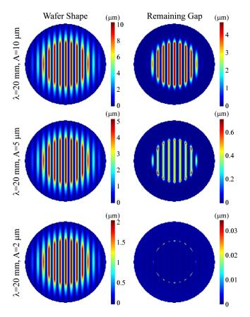
Fig. 3 Results of the 3-D finite element model for simulated wafer shapes with 1-D waviness in the center section. All results are shown for a clamping pressure of 80 kPa and a spatial wavelength of 20 mm.
