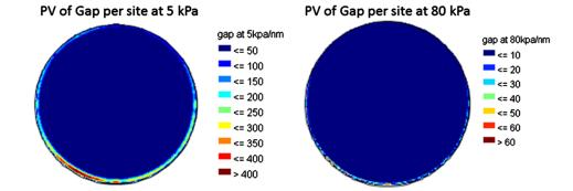
Fig. 7 Maps of the peak-to-valley (PV) of remaining gap per site ( $10 \times 10$  mm sites) for wafer 1 at 5 and 80 kPa. The wafer chucks nearly completely over the center of the wafer, but fails to chuck near the edges.
