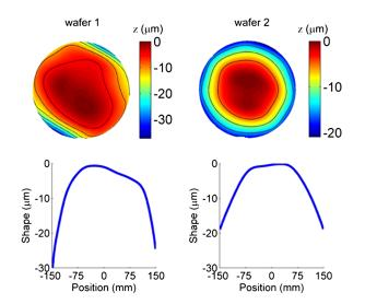
**Fig. 5** Top: Measured shape maps of two wafers, wafers 1 and 2, considered in 3-D finite element modeling. Contour lines (black) are shown at 5- $\mu$ m increments. Bottom: Profile of wafer shape along a line that passes through the center of the wafer and is oriented 45 deg from the horizontal. Note the higher-order wafer geometry features near the edge of wafer 1.
