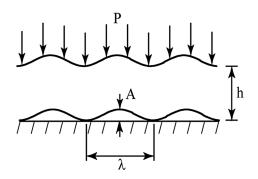
**Fig. 1** Schematic of wafer geometry and loading considered in the analytical and 2-D finite element models. The wafer has uniform thickness, *h*, and the medial-plane of the wafer varies sinusoidally with position in one dimension. As a result of this wafer shape, an initial gap with height, *A*, and wavelength,  $\lambda$ , exists between the elastic wafer and rigid chuck. The wafer is loaded uniformly with applied pressure, *P*.
