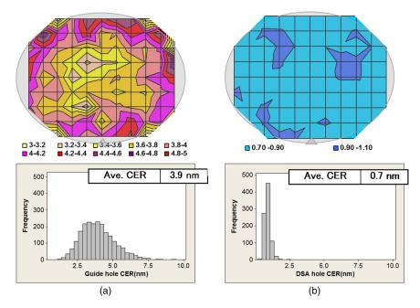
Fig. 9 Contact edge roughness of (a) prepattern and (b) DSA hole patterns on 300 mm wafer.
