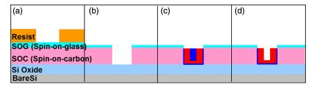
Fig. 1 Contact hole shrink process using graphoepitaxial DSAL (a) ArF lithography. (b) Stacked mask process RIE. (c) BCP coating and microphase separation. (d) Wet development.
