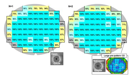
Fig. 10 Hole open yield on 300 mm wafers.
