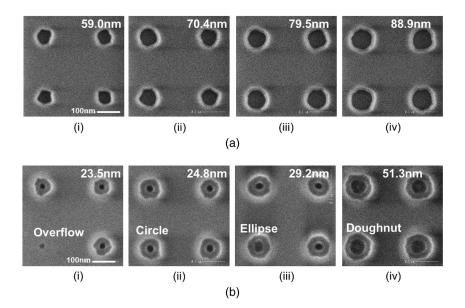
Fig. 3 SEM photomicrographs of the hole-type prepatterns and DSA holes (a) hole-type prepattern and (b) DSA holes.
