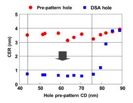
Fig. 5 Contact edge roughness of the hole-type prepattern and the DSA holes.
