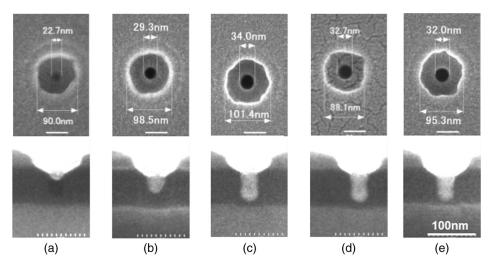
Fig. 2 Effect of DUV exposure dose on the PMMA cylindrical domain removal. Top-down and cross-sectional SEM images. Exposure doses are (a) 180 mJ/cm<sup>2</sup>, (b) 360 mJ/cm<sup>2</sup>, (c) 720 mJ/cm<sup>2</sup>, (d) 1080 mJ/cm<sup>2</sup>, and (e) 1800 mJ/cm<sup>2</sup>, respectively.
