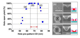
Fig. 6 Hole open yield dependence on hole prepattern CD.
