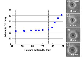
Fig. 4 Correlation between the hole-type prepattern critical dimension (CD) and the DSA hole CD.
