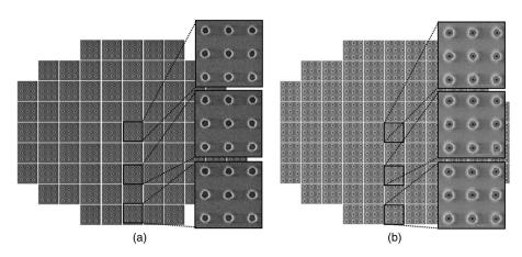
Fig. 7 Top-down SEM images of (a) prepattern and (b) DSA hole patterns on 300 mm wafer.
