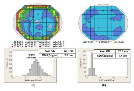
Fig. 8 CD uniformity of (a) prepattern and (b) DSA hole patterns on 300 mm wafer.
