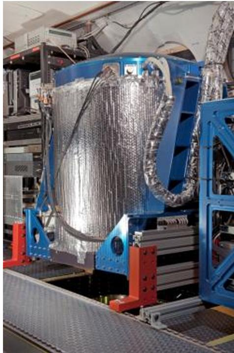
**Fig. 2** The Doppler aerosol wind lidar instrument installed inside the UC-12B aircraft. A cylindrical enclosure houses the laser and optical receiver.
