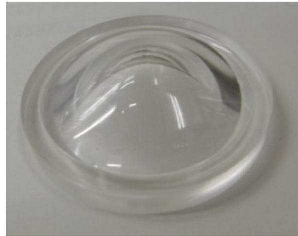
**Fig. 11** Photograph of the actual turned aspherical lens.
