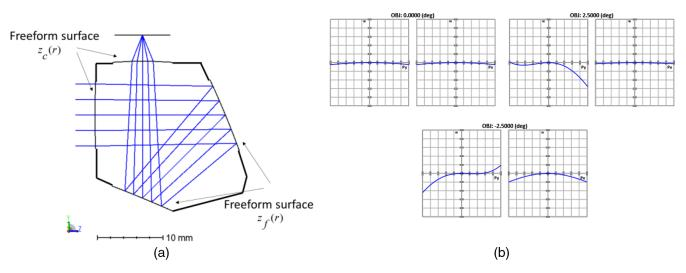
**Fig. 12** The starting design of a monolithic free-form objective is constructed with confocal surfaces. (a) Layout and (b) OPD plots (the plot scale is 5 waves at 9  $\mu$ m). Combination of free-form surfaces  $z_f(r)$  and  $z_c(r)$  allows to achieve stigmatic imaging on-axis surface after surface.
