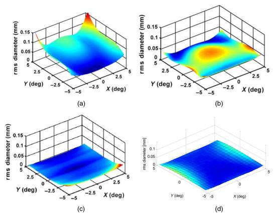
**Fig. 10** The RMS Spot Size over the field of the three-mirror system. (a) The design with conventional aspheric surfaces reported by Chrisp, (b) the design with *XY* polynomial surfaces reported by Chrisp, (c) the design with NURBS free-form surfaces reported by Chrisp, and (d) the current design with aspherical surfaces  $z_f(r)$ .
