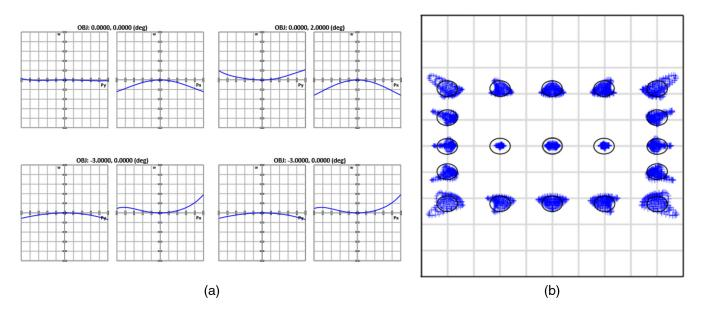
**Fig. 6** Imaging performance of the final two-mirror unobscured Schwarzschild-type telescope design. (a) OPD plots (plot scale is 1 wave at 0.550  $\mu$ m) and (b) full-field spot diagram at 0.550  $\mu$ m. Close to diffraction limited performance over an FOV of 6 × 4 deg was achieved.
