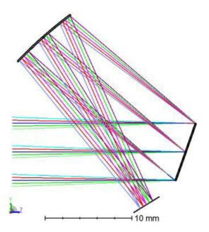
Fig. 5 Layout of the final two-mirror unobscured Schwarzschild-type telescope design. Aspheric polynomial terms are used to correct off-axis aberrations.
