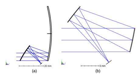
**Fig. 3** The elements are tilted and/or decentered to generate an unobscured optical system. Mirror surfaces are defined with (a) standard axially symmetric conic surfaces and (b) aspheric/free-form surfaces  $z_f(r)$ .
