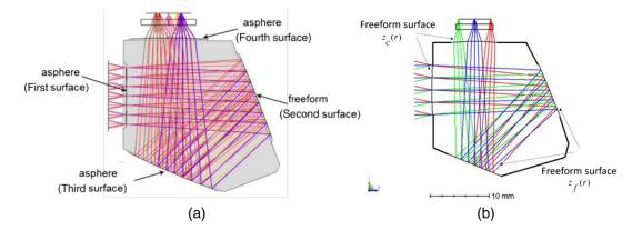
**Fig. 13** Layout of the monolithic objective design. (a) The design with aspheric and Zernike free-form surfaces reported by Kiontke and (b) the current design with aspherical/free-form surfaces  $z_f(r)$  and  $z_c(r)$ . In the current design, aspheric polynomials are used to correct off-axis aberrations.
