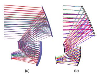
**Fig. 8** Layout of the three-mirror telescope. (a) The design with NURBS free-form surfaces reported by Chrisp; (b) the current design with aspherical/free-form surfaces  $z_f(r)$ . In the current design, up to eighth-order plane-symmetric polynomials are used to correct off-axis aberrations.
