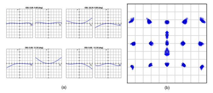
Fig. 14 Imaging performance of the final monolithic objective design. (a) OPD plots (the plot scale is 1 wave at 9  $\mu$ m) and (b) spot diagrams at 9  $\mu$ m. Excellent, balanced performance over an FOV of 37 × 25 deg was achieved.
