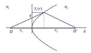
Fig. 11 Geometrical variables used to define the Cartesian oval surface. All rays from the object point O to the image point O' have equal optical path length.
