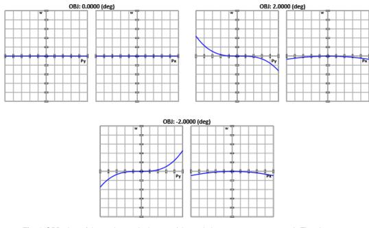
Fig. 4 OPD plots of the unobscured telescope (plot scale is two waves at 0.550  $\mu$ m). The plane-symmetric system designed with confocal surfaces performs close to the corresponding axially symmetric system.
