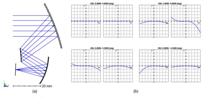
**Fig. 7** The starting design of a three-mirror telescope is constructed with confocal surfaces. (a) Layout and (b) OPD plots (the plot scale is 10 waves at 3  $\mu$ m). In this design, imaging on-axis is stigmatic surface after surface. Tilt of the tertiary mirror is adjusted to correct field tilt and linear astigmatism.
