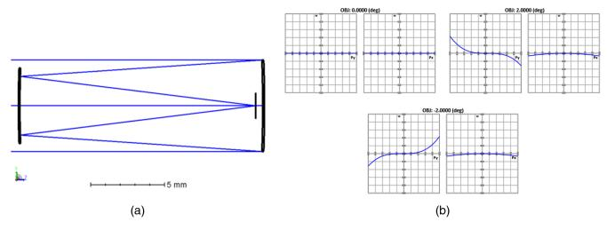
**Fig. 2** The starting design of a two-mirror unobscured Schwarzschild-type telescope. (a) Layout and (b) OPD plots (plot scale is 2 waves at 0.550  $\mu$ m). In this design, imaging on-axis is stigmatic surface after surface.
