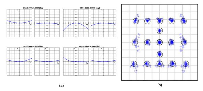
**Fig. 9** Imaging performance of the final three-mirror telescope. (a) OPD plots (the plot scale is 1 wave at 3  $\mu$ m) and (b) spot diagrams at 3  $\mu$ m. Close to diffraction limited performance over an FOV of 10 × 9 deg was achieved.
