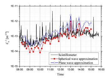
**Fig. 17** The structure parameter  $C_n^2$  of the refractive index measured by the Scintec BLS 900 scintillometer and by the angle-of-arrival-fluctuations method.
