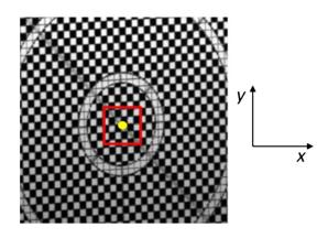
Fig. 2 Image of the loudspeaker membrane recorded with the high-speed camera. The red rectangle marks the subset used for the calculations, the yellow point the investigated pixel.
