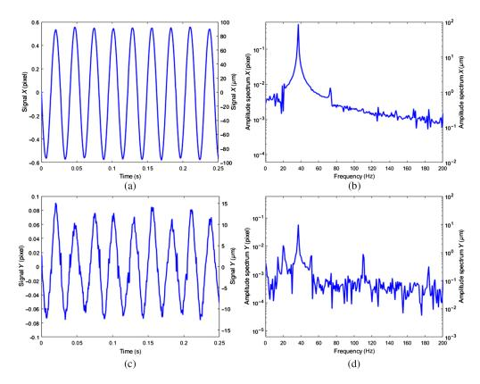
**Fig. 3** (a)–(d) Vibration measurement using the high-speed imaging technique. Subpixel displacement over the time along the x and y axes and the corresponding Fourier spectra.
