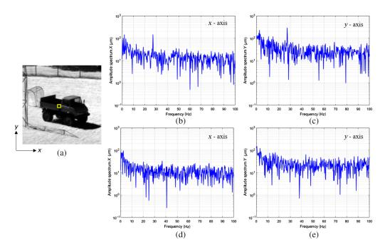
**Fig. 12** Infrared image of the small truck recorded with the InGaAs camera in the spectral range 0.9 to 1.7  $\mu$ m (a) and the vibrational spectra acquired from the position marked by the yellow square with (b), (c) engine on and (d), (e) engine off.
