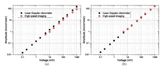
**Fig. 4** Vibration amplitude of the loudspeaker membrane as a function of applied signal: (a) before and (b) after the angle correction. The red points show the measurements with the high-speed camera, the black points those with the LDV.
