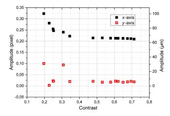
Fig. 6 Measured vibration amplitude as a function of modulation contrast for the investigated subset.
