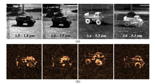
**Fig. 14** (a) Sample images and (b) corresponding 2D vibration signatures of the idling engine small truck recorded with the HgCdTe camera in various spectral ranges at the engine main frequencies between 27 and 29 Hz.
