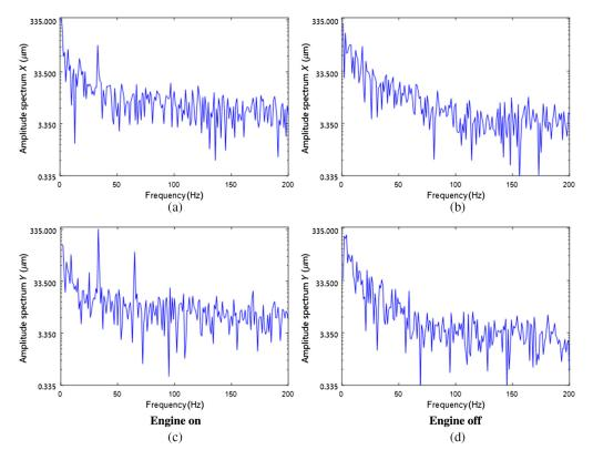
Fig. 8 High-speed camera: vibrational spectra of the small truck acquired from the position marked by a red square at Fig. 7(b) [(a), (c) engine on and (b), (d) engine off].
