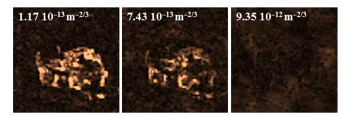
**Fig. 18** 2D vibration signature of the idling engine small truck recorded with the InGaAs camera in the spectral range 0.9 to 1.7  $\mu$ m under different turbulent conditions. The inserted values give the determined  $C_n^2$ .
