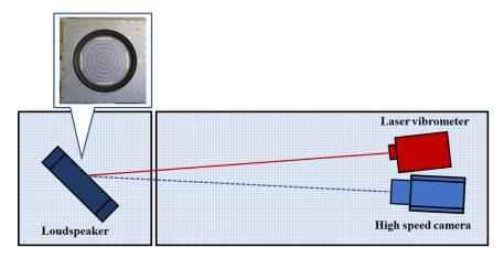
Fig. 1 Experimental setup for optical measurement of loudspeaker vibration in comparison with LDV.
