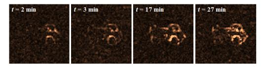
**Fig. 15** 2D vibration signature of the idling engine small truck recorded with the HgCdTe camera in the spectral range 4.8 to 5.3  $\mu$ m for different engine run time durations.
