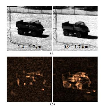
**Fig. 13** (a) Sample images and (b) corresponding 2D vibration signatures of the idling engine small truck recorded with the InGaAs camera in two spectral ranges at the engine main frequencies of 27.25 and 26.25 Hz, respectively.
