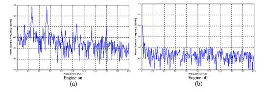
Fig. 10 LDV: vibrational spectra of a small truck [with (a) engine on and (b) engine off] acquired from an arbitrary position marked by a white circle at Fig. 11.
