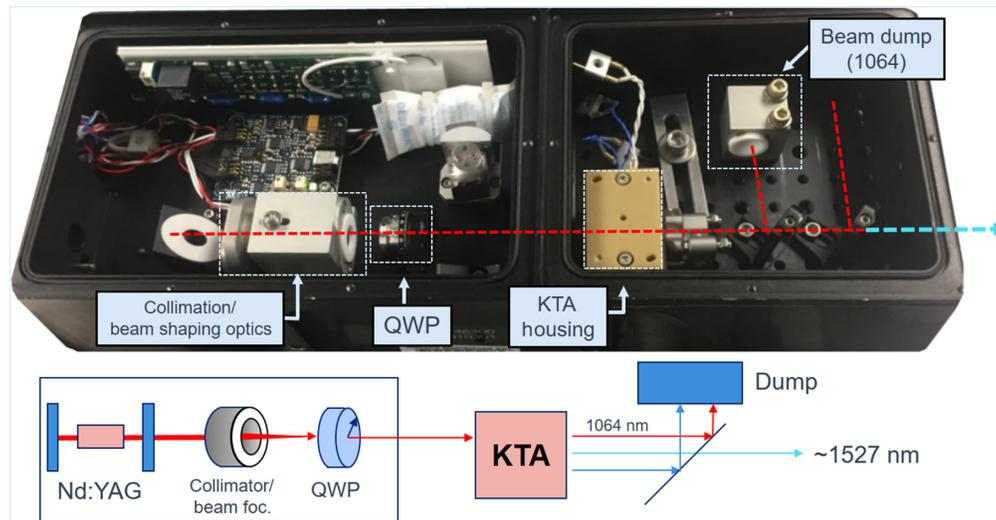
**Fig. 2** Quantel CFR 300—postmodification for operation at 1527 nm—resulting in  $\approx 85$  mJ at up to 28 Hz.
