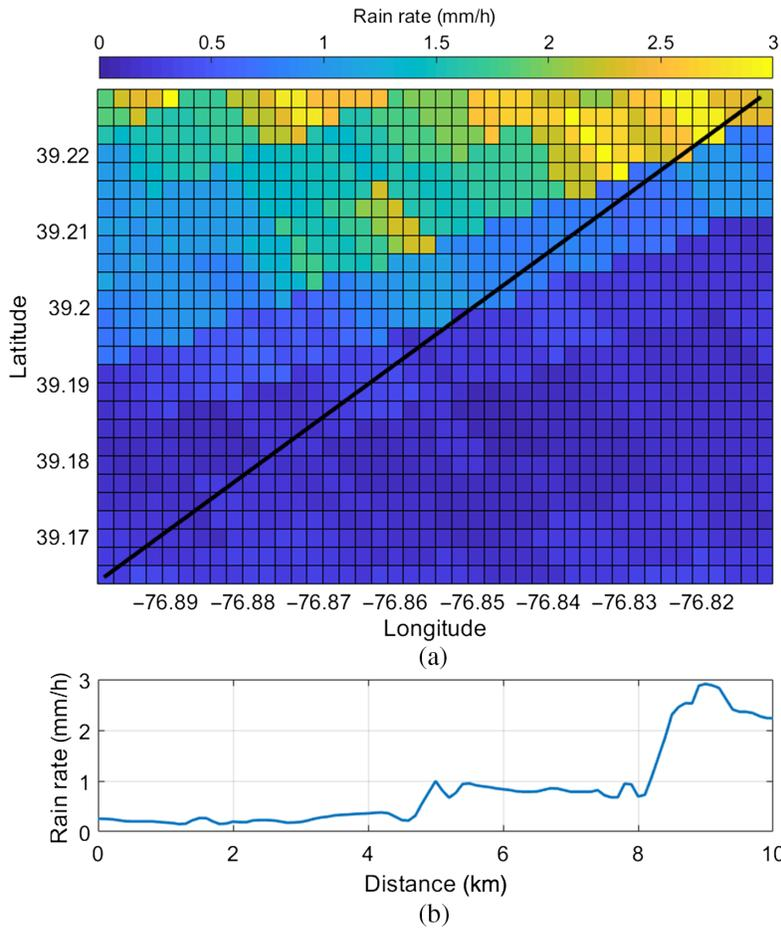
**Fig. 8** (a) NEXRAD derived rain rate (mm/h) during the time of the test. The bold black line is the LoS from the transmitter to the water tower. (b) Rain rate (mm/h) along the line-of-sight. A path weighted average rain rate of 0.83 mm/h was calculated and used to seed Modtran.
