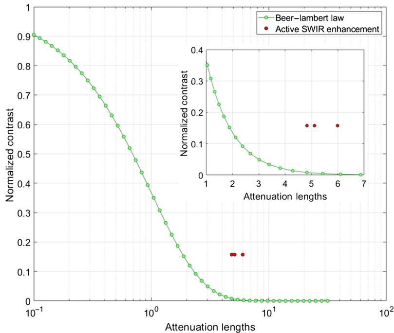
**Fig. 11** Normalized contrast as a function of attenuation lengths for Beer–Lambert law evaluated at  $\lambda = 1527$  nm and calculated normalized contrast of the range-gated imager. Normalized contrast of the imager was found to be 0.145 and is plotted for a 10-km range for each of the extinction values in Table 1. Inset: linear scale (attenuation length =  $\sigma_{\text{ext}} \times \text{range}$ ).
