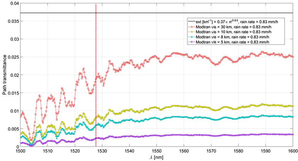
**Fig. 9** One-way 10-km path transmittance from the laser source to the water tower. Top black curve is the transmittance solely due to the rain at 0.83 mm/h. The four color curves are the results of MODTRAN with the rain rate fixed and different visibilities. The dashed-red vertical line is the operational laser wavelength.
