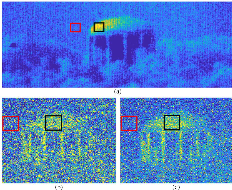
**Fig. 10** (a) Clear day image of water tower used to calculate contrast for normalization metric; (b) single frame from range gated imager through rain; and (c) 10-frame average from range gated imager. Black boxes represent the regions where the background and signal were determined for the contrast calculation. The red box was used for the background and the black box on the tower was utilized for the signal.
