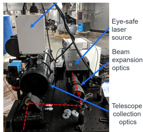
**Fig. 3** SWIR active imaging integrated system. Laser path shown in red. The laser source was co-aligned with the collection optics, going out behind the secondary mirror of the imager.
