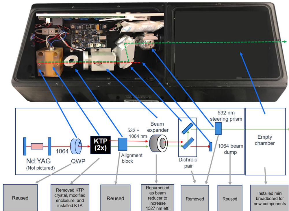
**Fig. 1** Quantel CFR 300 as delivered. Many parts were repurposed and reused to maintain the laser operation within the original housing.
