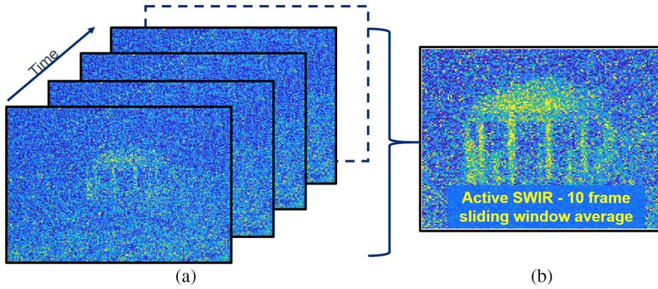
**Fig. 7** Active SWIR images during the rain penetration test. (a) A single frame (500-ns exposure) and (b) a typical 10-frame sliding window average.
