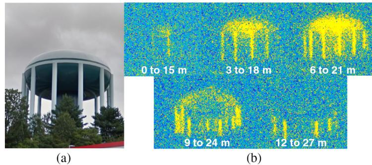
**Fig. 4** (a) Water tower imaged locally from the ground  $\approx 30$  m in diameter. (b) Depth map of water tower as collected from the rooftop at JHU-APL at a 10-km range utilizing the range gated imager. The imager's exposure time was set to 100 ns and stepped by 20 ns to image the water tower from front to back. The 0- to 15-m exposure shows primarily the front support struts, whereas the 12- to 27-m exposure shows the rear supports.
