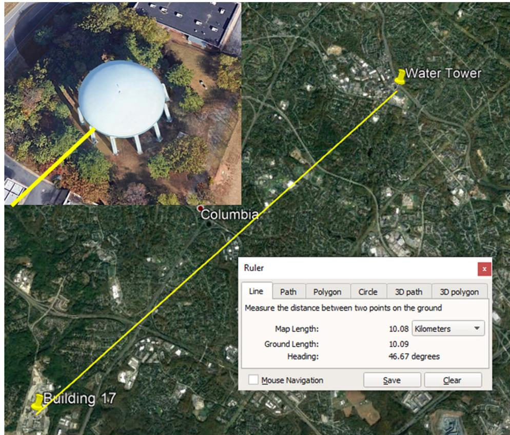
**Fig. 5** Satellite image of the 10-km path from JHU/APL's facility to the water tower. Inset: zoomed image of the water tower with the line-of-sight marked in yellow. The water tower has a diameter of 30 m.
