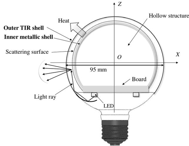
**Fig. 3** Schematic cross-sectional view of concentric shells composed of outer TIR shell and inner metallic shell for large globe LED bulb with outermost diameter of 95 mm. The cross-sectional plane is set to  $X$ - $Z$  plane in a global Cartesian coordinate system  $(X, Y, Z)$ . The center of the concentric shells corresponds to the global coordinate origin  $O$ . The LEDs are axisymmetrically arranged around the  $Z$  axis where their emitting surfaces face in the negative  $Z$  direction.
