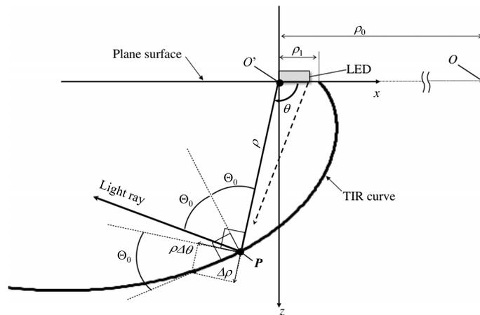
**Fig. 4** Schematic cross-sectional view close to an LED in  $x$ - $z$  plane of a local coordinate system  $(x, y, z)$  with its origin  $O'$ . The origin  $O'$  corresponds to an edge of the LED emitting surface. A 2D polar coordinate system  $(\rho, \theta)$  is also taken with its origin corresponding to the  $O'$ .
