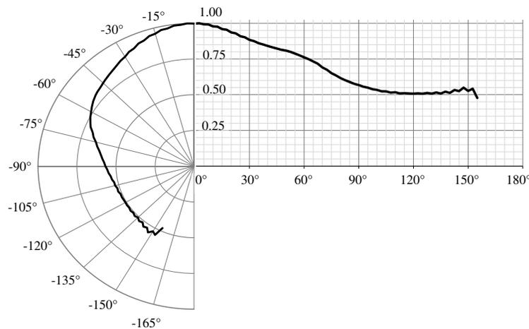
**Fig. 7** Measured light angle distribution of the fabricated prototype of the large globe LED bulb. Solid line denotes experimental result. The range of angle is from  $-180$  deg to 0 deg on the left, and from 0 deg to  $+180$  deg on the right.
