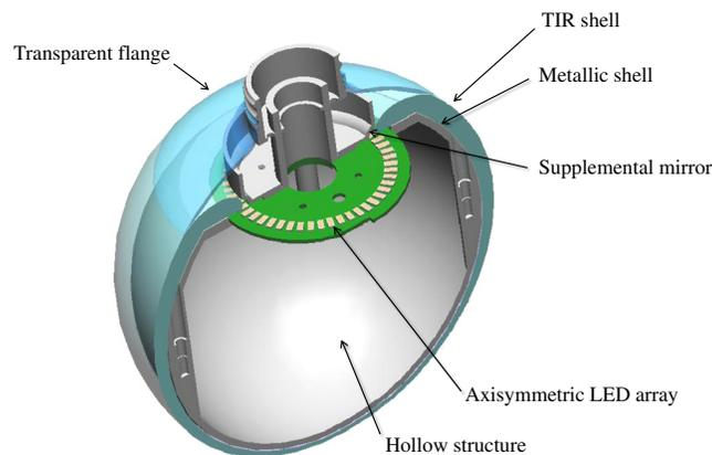
**Fig. 5** Perspective view of half cut of light LED bulb prototype with large globe diameter of 95 mm using the concentric shells composed of TIR shell and metallic shell. Axisymmetric LED array is composed of multiple LEDs. Supplemental mirror is introduced to reflect some of the light rays emitted from the LEDs into the TIR shell. Transparent flange is attached to protect the LEDs from dust. Hollow structure can be constructed by concentric shells, which can accommodate several devices.
