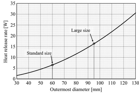
**Fig. 2** Calculated heat release rate  $Q$  [W] using Eq. (1) with respect to outermost diameter of  $2R_{\text{TIR}}$  of concentric shells. The outermost diameters of standard-size and large-size bulbs are 60 and 95 mm, respectively.
