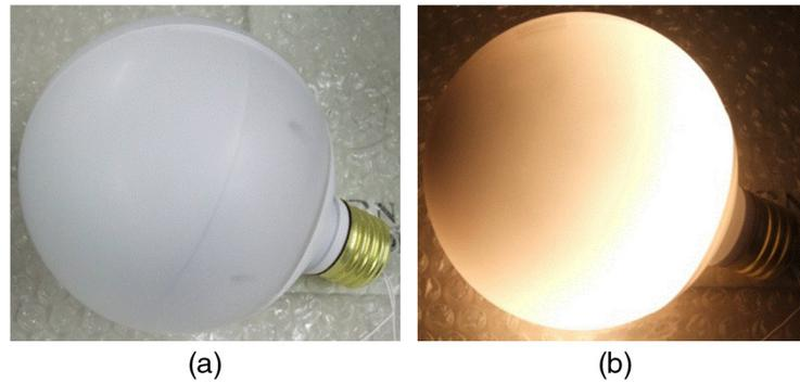
**Fig. 8** Fabricated prototype of large globe LED bulb composed of concentric shells where the outermost surface is sandblasted. (a) The LED bulb turned off and (b) turned on.
