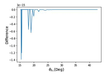
**Fig. 1** Difference between the full BRDF (un-normalized) functions when  $\theta_i$  and  $\sigma_g$  are kept constant at 40 deg and 0.1 deg, respectively and  $\phi_s$  is varied from  $3\pi/4$  to  $5\pi/4$  (in radians). As one can see, the difference is minimal, on the order of  $10^{-15}$ , which is likely due to computational rounding error in the trigonometric functions.
