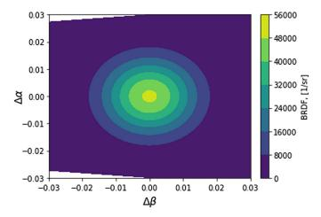
**Fig. 2** Simulated isotropic BRDF data for  $\sigma_g = 0.005$  and  $\theta_i = 20^\circ$ . The average eccentricity was  $0.897 \pm 0.006$  for this particular  $\theta_i$ , indicating that the eccentricity of contours remains relatively low (near circular) as well as constant for isotropic BRDFs.
